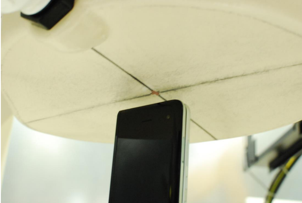
SAR Test Setup Photo 11 – Closed Configuration Top Edge at 1.0cm
