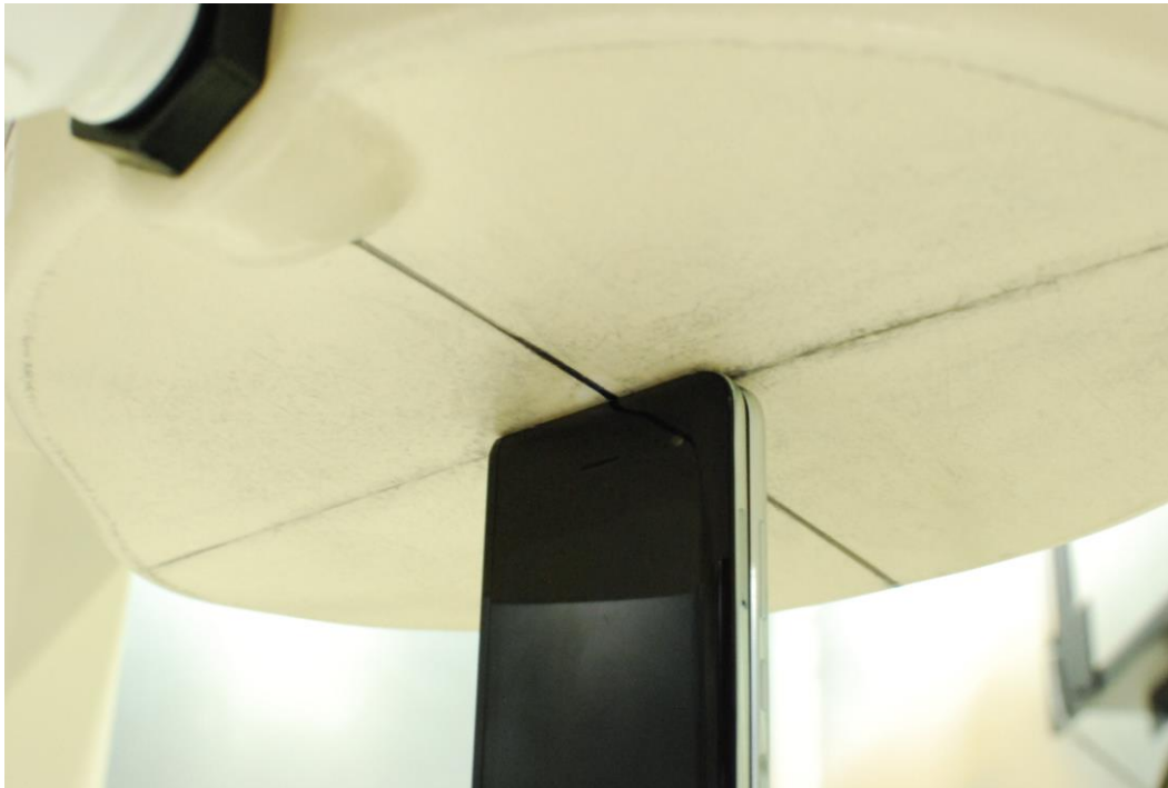
SAR Test Setup Photo 12 – Closed Configuration Top Edge at 0.0cm
