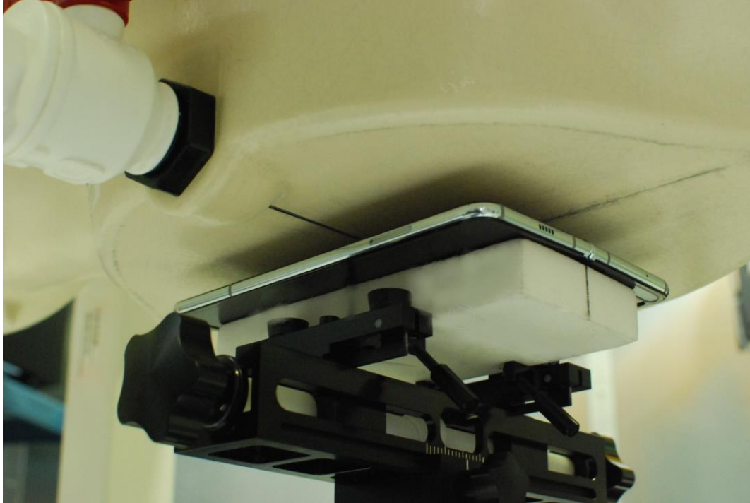
SAR Test Setup Photo 19 – Open Configuration Back Side at 1.0cm
