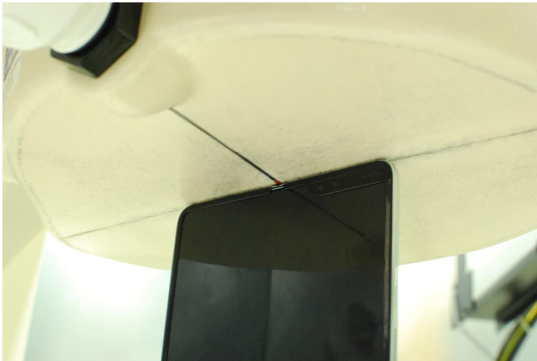
SAR Test Setup Photo 26 – Open Configuration Top Edge at 0.0cm
