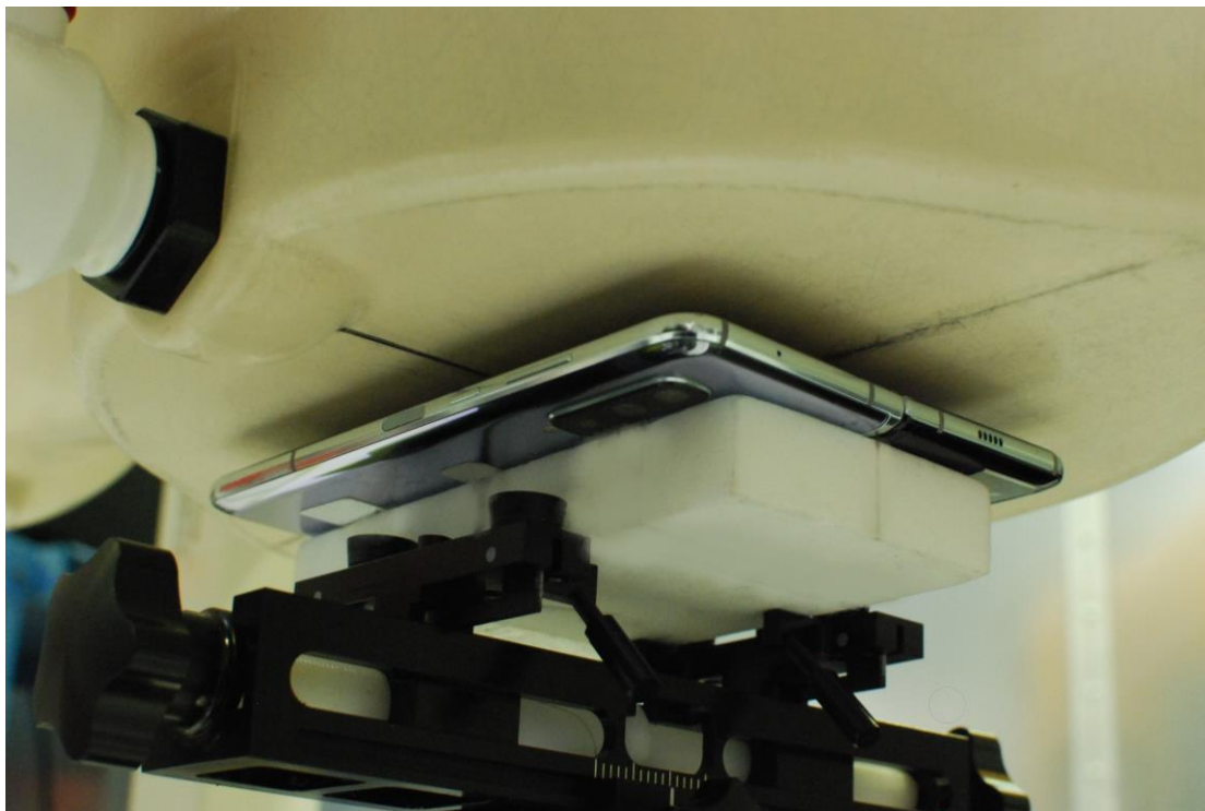
SAR Test Setup Photo 22 – Open Configuration Front Side at 1.0cm
