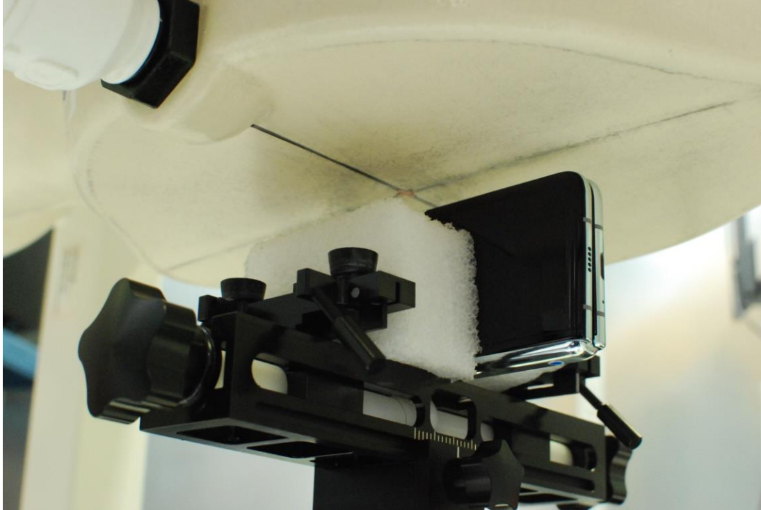
SAR Test Setup Photo 15 – Closed Configuration Right Edge at 1.0cm
