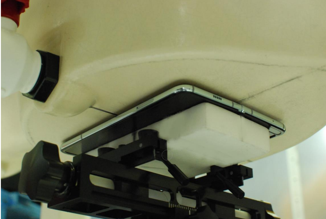
SAR Test Setup Photo 21 – Open Configuration Back Side at 0.0cm
