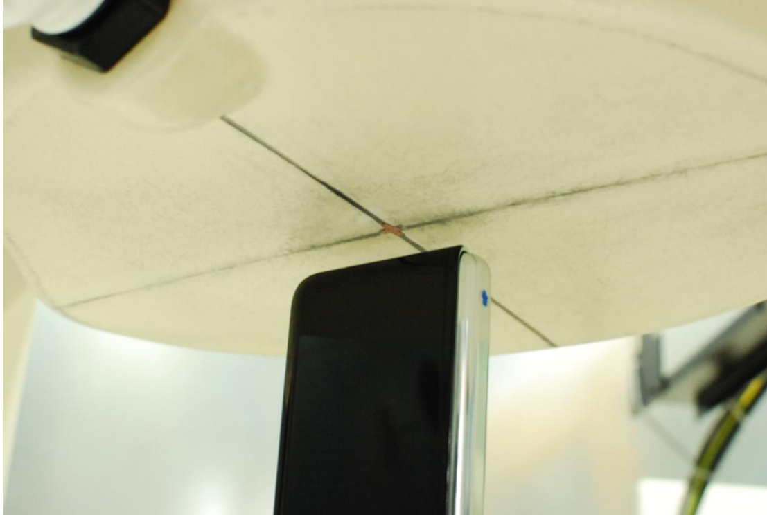
SAR Test Setup Photo 13 – Closed Configuration Bottom Edge at 1.0cm
