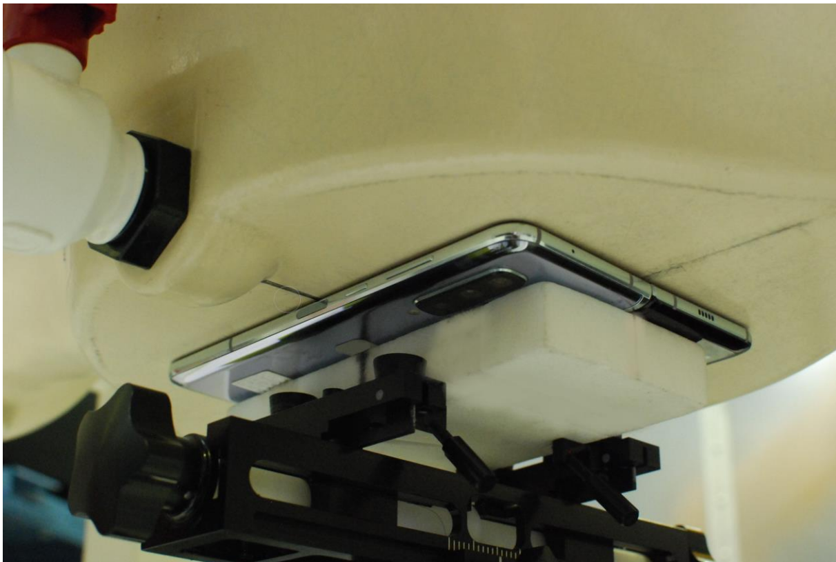
SAR Test Setup Photo 24 – Open Configuration Front Side at 0.0cm
