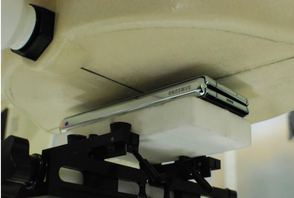
SAR Test Setup Photo 7 – Closed Configuration Back Side at 0.6 cm
