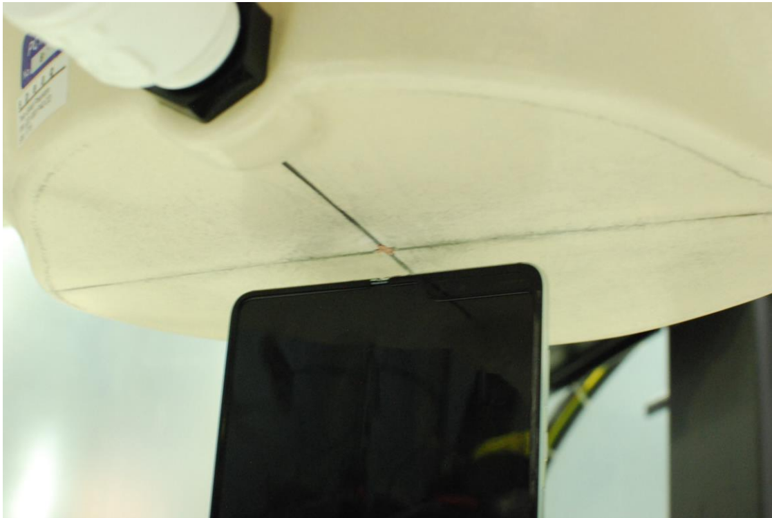
SAR Test Setup Photo 25 – Open Configuration Top Edge at 1.0cm
