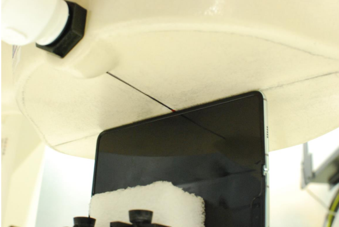
SAR Test Setup Photo 31 – Open Configuration Right Edge at 0.0cm
