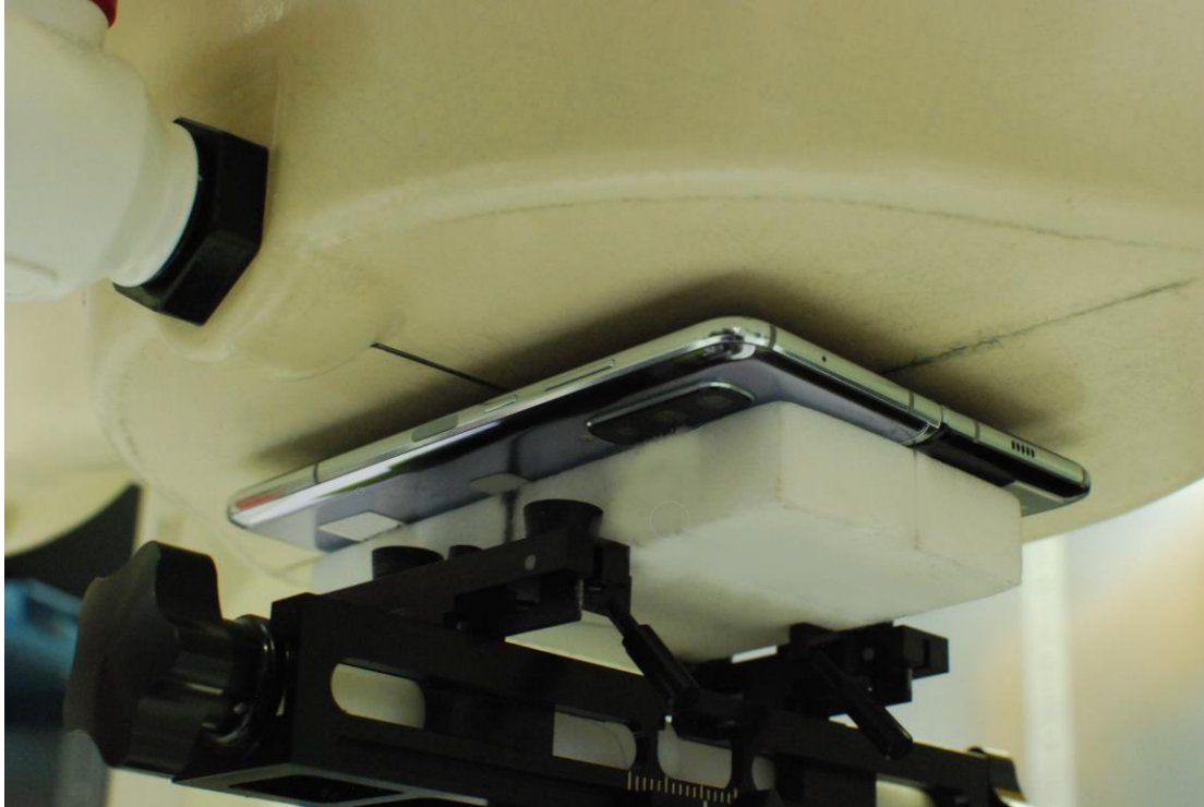
SAR Test Setup Photo 23 – OpenConfiguration Front Side at 0.7cm
