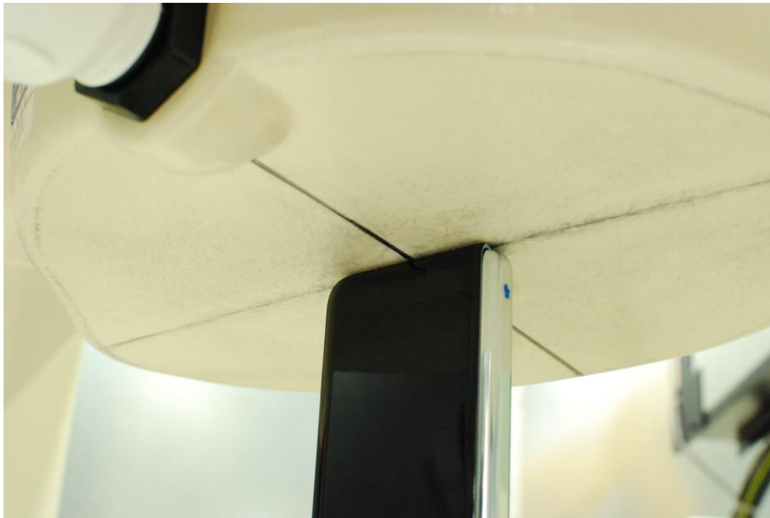
SAR Test Setup Photo 14 – Closed Configuration Bottom Edge at 0.0cm
