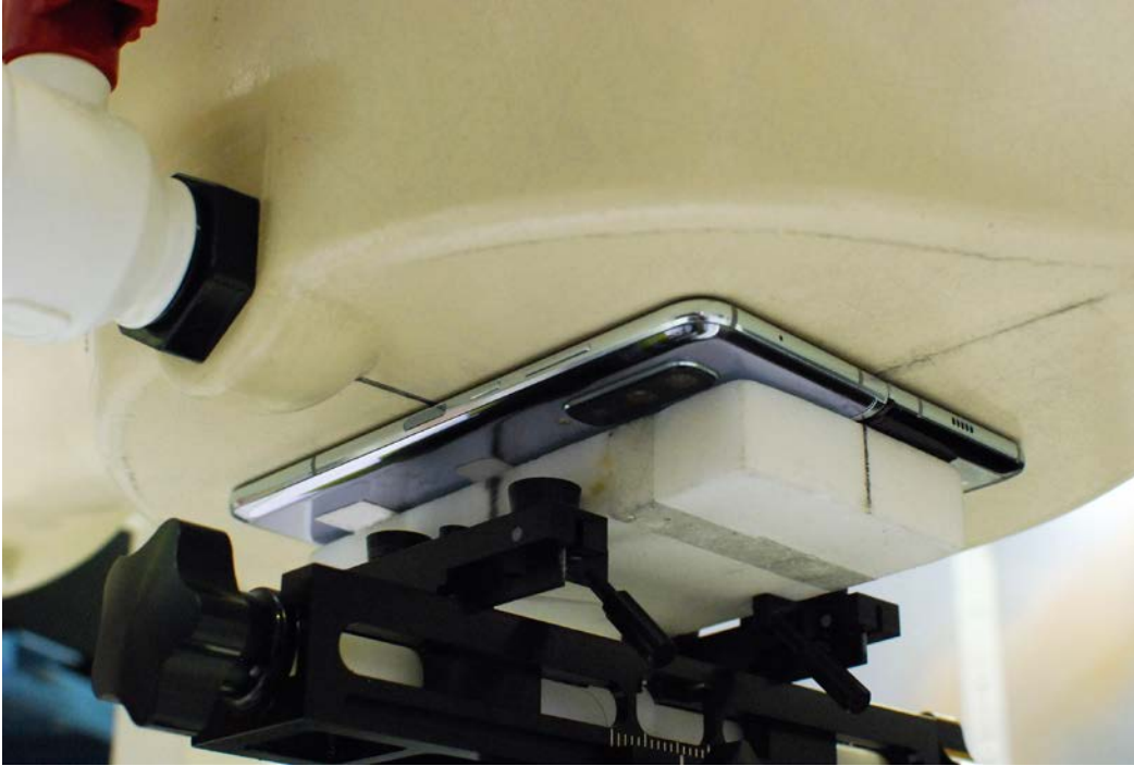
SAR Test Setup Photo 25 – Open Configuration Front Side at 0.0 cm
