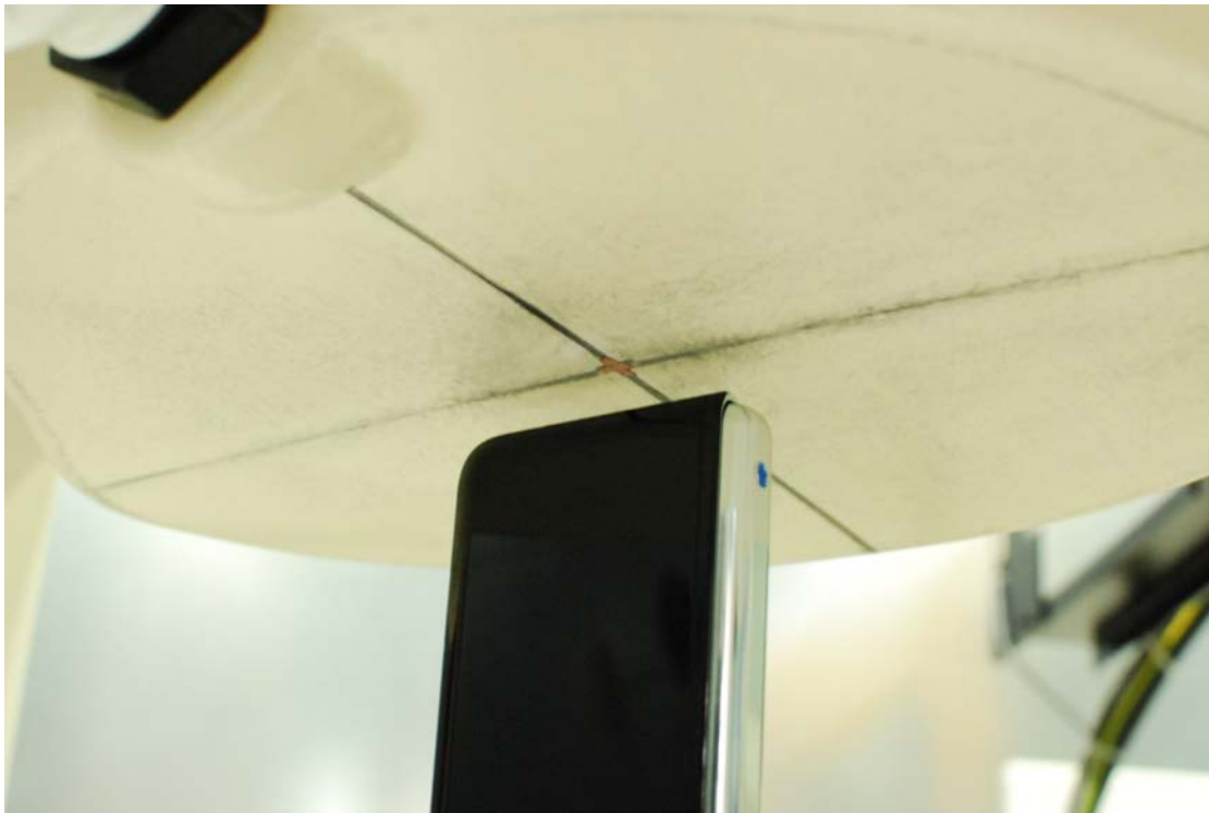
SAR Test Setup Photo 14 – Closed Configuration Bottom Edge at 1.0 cm
