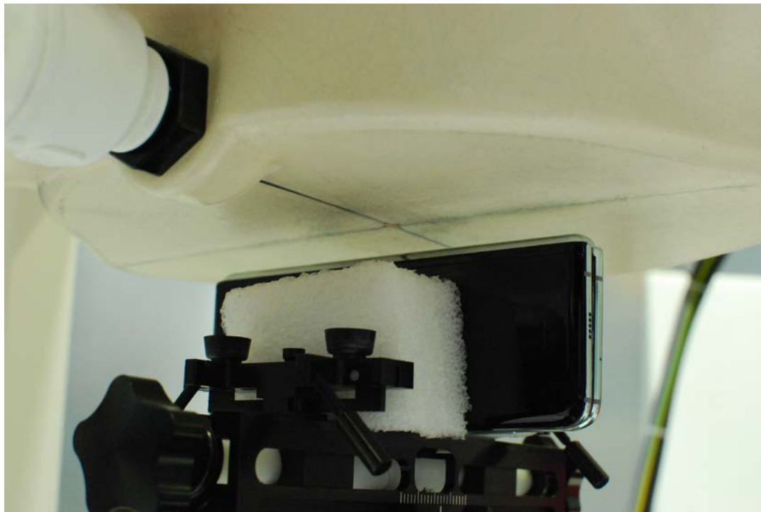
SAR Test Setup Photo 18 – Closed Configuration Left Edge at 1.0cm
