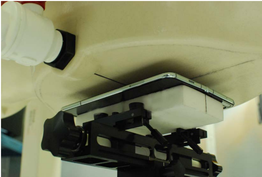
SAR Test Setup Photo 20 – Open Configuration Back Side at 1.0cm
