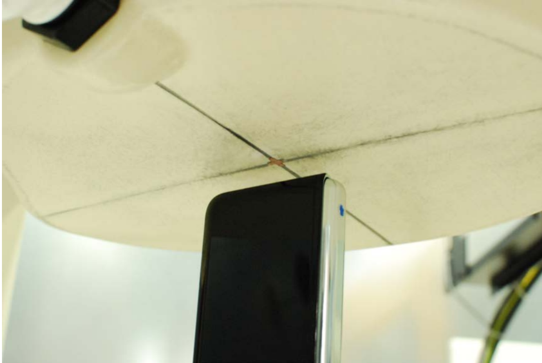
SAR Test Setup Photo 13 – Closed Configuration Bottom Edge at 1.1 cm
