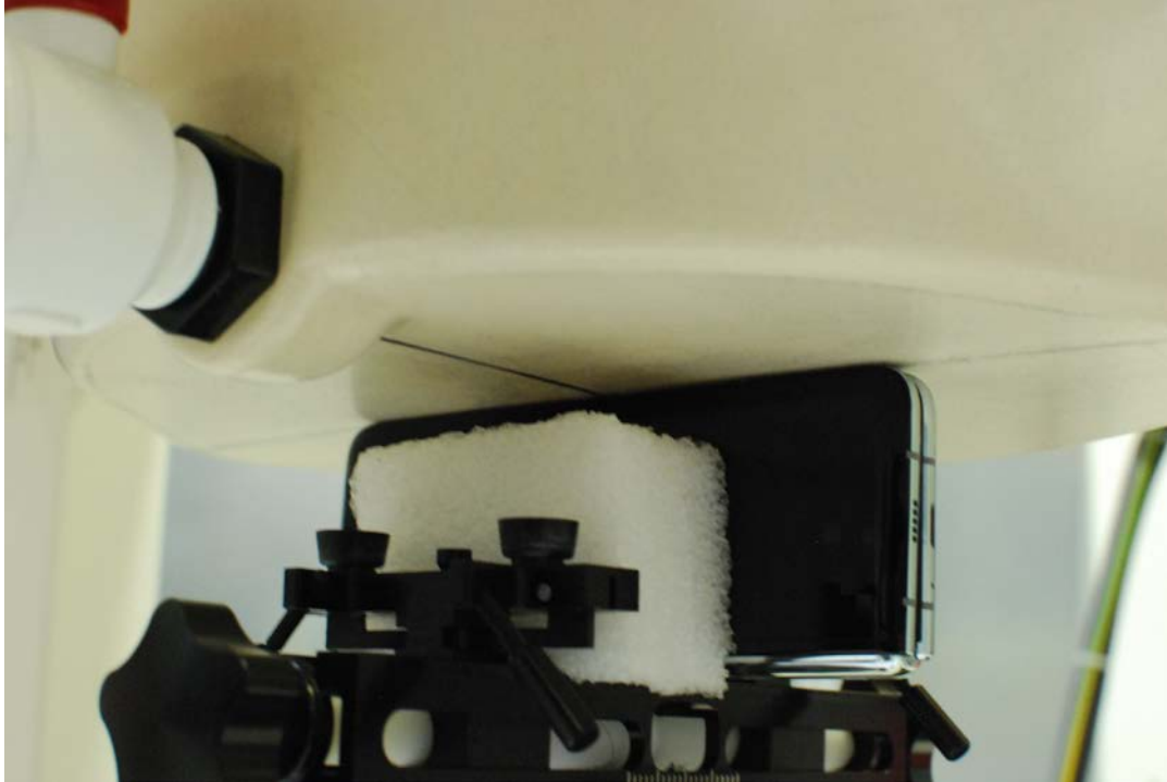
SAR Test Setup Photo 17 – Closed Configuration Right Edge at 0.0cm
