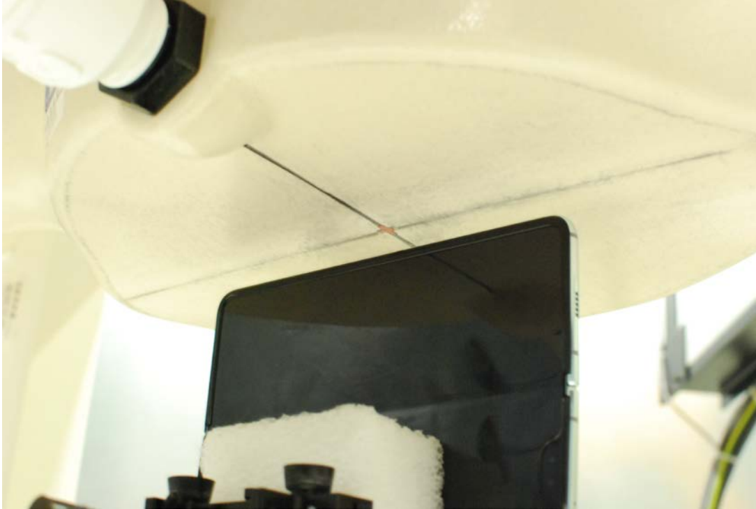
SAR Test Setup Photo 31 – Open Configuration Right Edge at 1.0 cm
