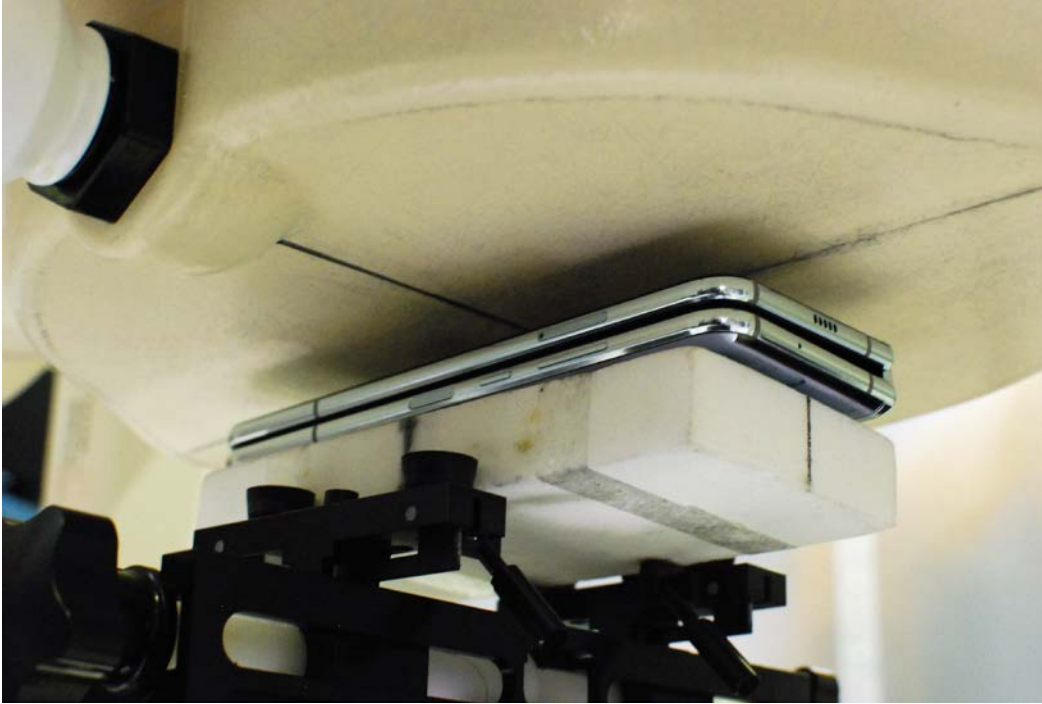
SAR Test Setup Photo 9 – Closed Configuration Front Side at 1.0 cm
