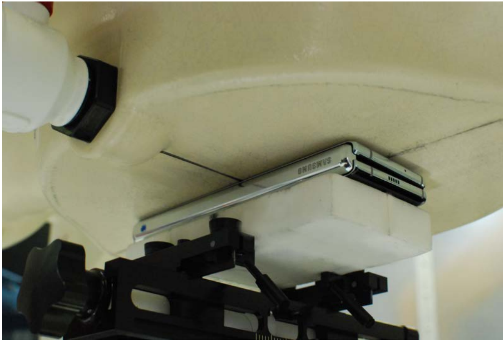
SAR Test Setup Photo 8 – Closed Configuration Back Side at 0.0 cm
