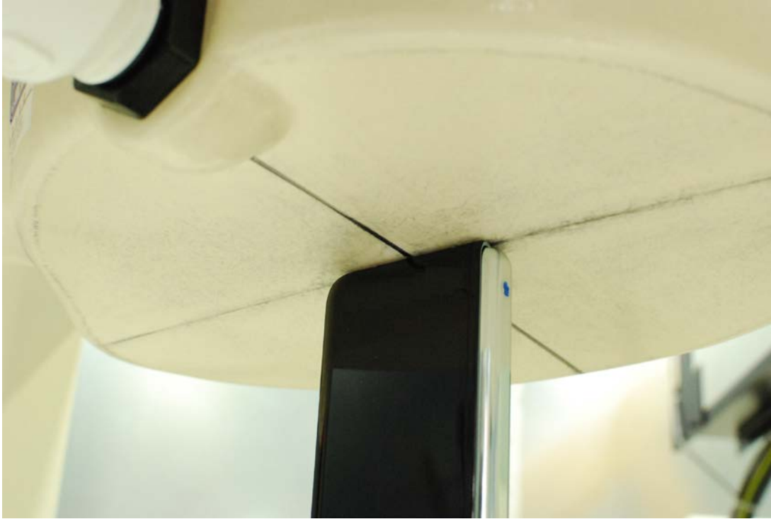
SAR Test Setup Photo 15 – Closed Configuration Bottom Edge at 0.0 cm
