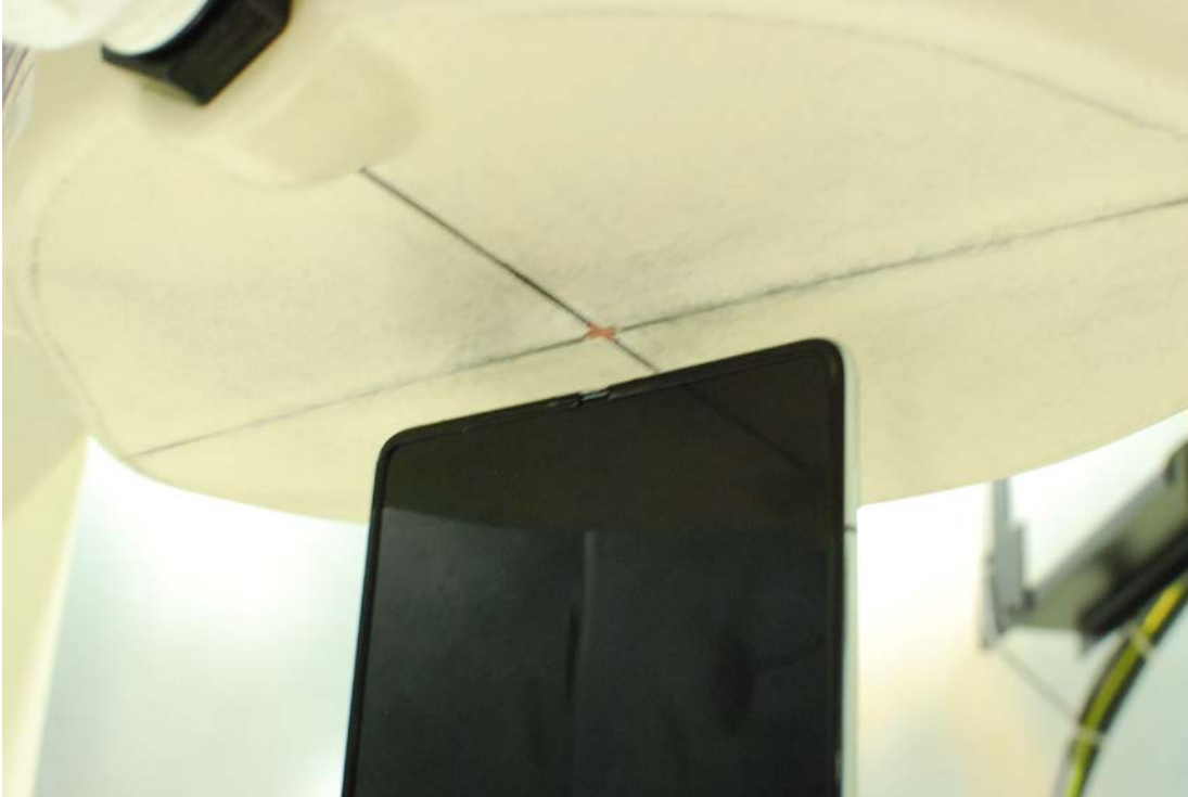
SAR Test Setup Photo 29 – Open Configuration Bottom Edge at 1.0 cm
