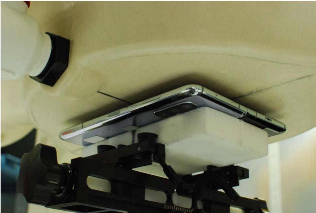
SAR Test Setup Photo 24 – Open Configuration Front Side at 0.8 cm
