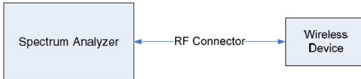
Figure 7-1. Test Instrument & Measurement Setup
