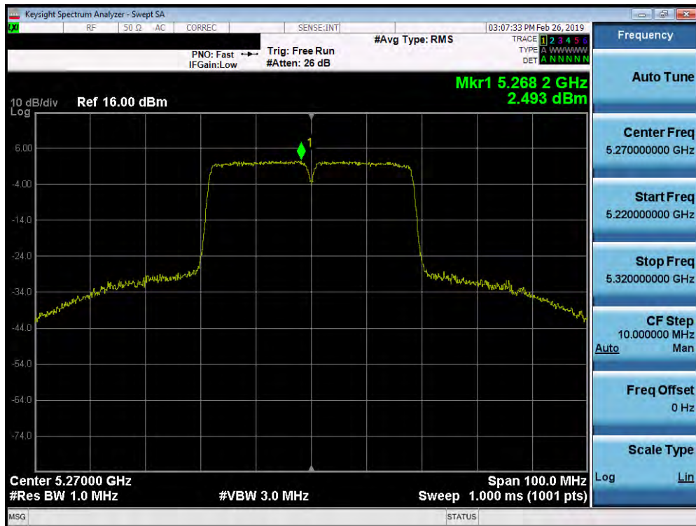
Plot 7-223. Power Spectral Density Plot SISO ANT2 (40MHz BW 802.11n (UNII Band 2A) – Ch. 54)
