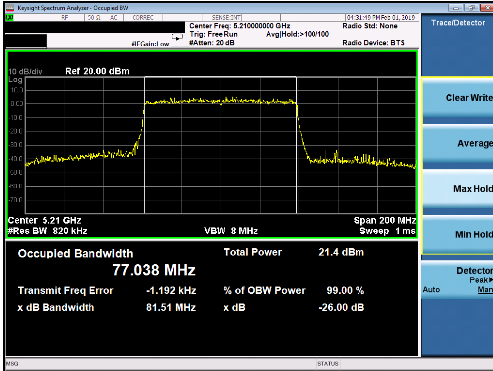
Plot 7-66. 26dB Bandwidth Plot SISO ANT2 (80MHz BW 802.11ax (UNII Band 1) – Ch. 42)
