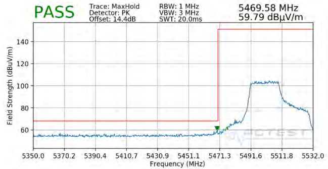
Plot 7-443. Radiated Lower Band Edge Plot SISO ANT2 (Peak – UNII Band 2C – 242 Tones)
