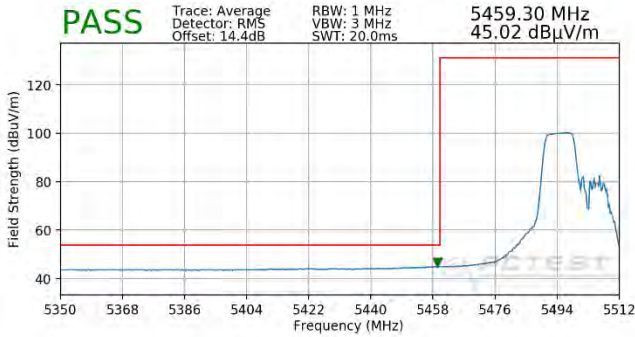
Plot 7-386. Radiated Lower Band Edge Plot SISO ANT1 (Average – UNII Band 2C – 106 Tones)
