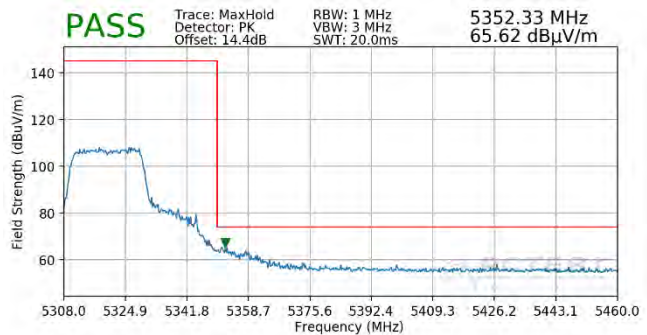
Plot 7-420. Radiated Upper Band Edge Plot SISO ANT2 (Peak – UNII Band 2A – 242 Tones)
