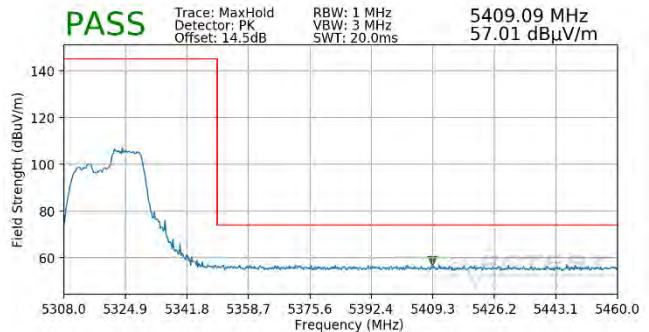
Plot 7-385. Radiated Upper Band Edge Plot SISO ANT1 (Peak – UNII Band 2A – 106 Tones)
