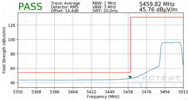
Plot 7-379. Radiated Lower Band Edge Plot SISO ANT1 (Average – UNII Band 2C – 242 Tones)
