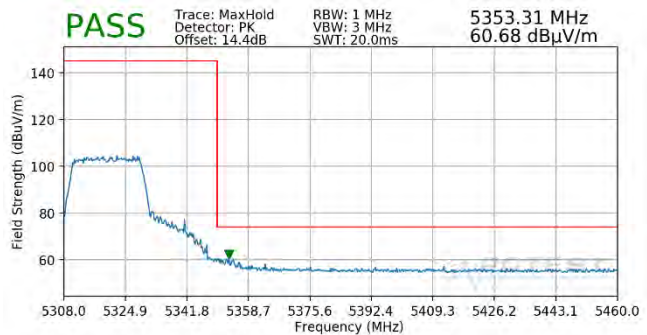
Plot 7-378. Radiated Upper Band Edge Plot SISO ANT1 (Peak – UNII Band 2A – 242 Tones)
