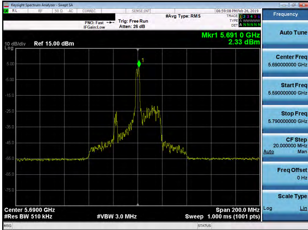
Plot 7-264. Power Spectral Density Plot MIMO ANT2 (80MHz BW 802.11ax – 26 Tones (UNII Band 2C) – Ch. 138)
