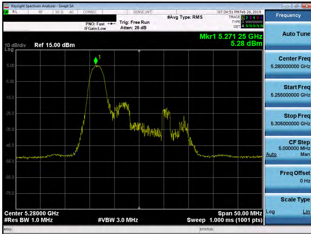
Plot 7-224. Power Spectral Density Plot MIMO ANT1 (20MHz BW 802.11ax – 26 Tones (UNII Band 2A) – Ch. 56)
