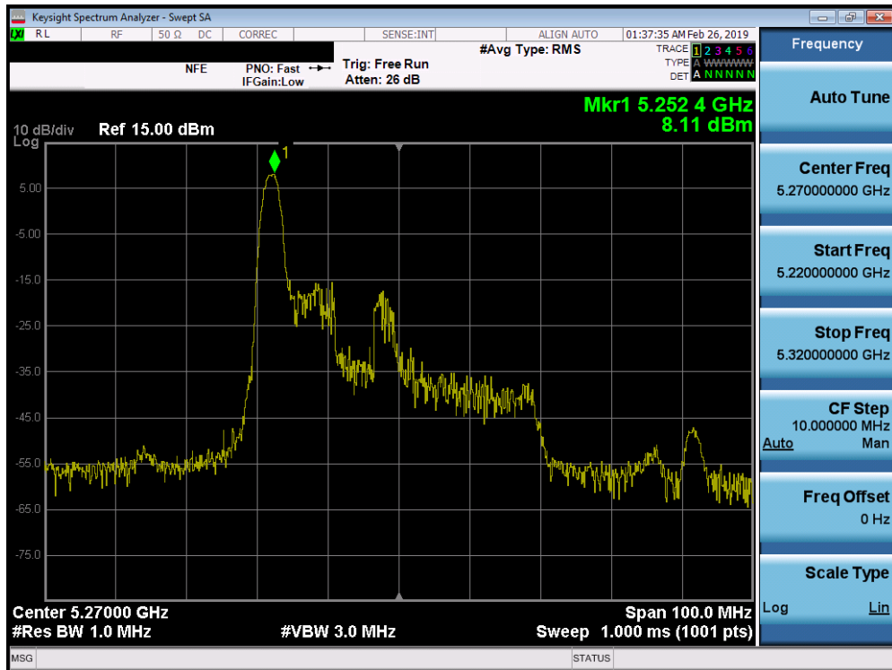
Plot 7-118. Power Spectral Density Plot SISO ANT1 (40MHz BW 802.11ax – 26 Tones (UNII Band 2A) – Ch. 54)
