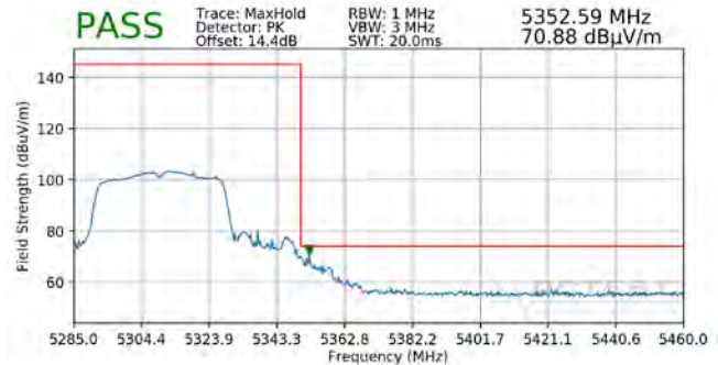
Plot 7-317. Radiated Upper Band Edge Plot SISO ANT1 (Peak – UNII Band 2A)
