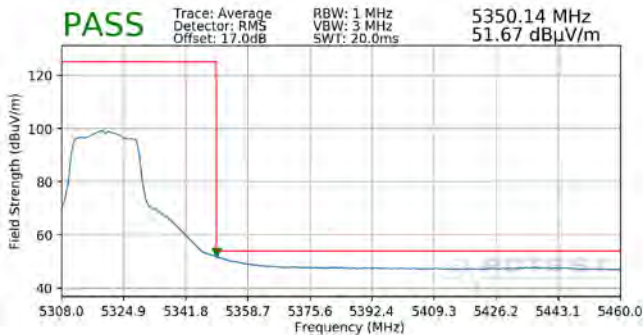
Plot 7-353. Radiated Upper Band Edge Plot MIMO (Average – UNII Band 2A)
