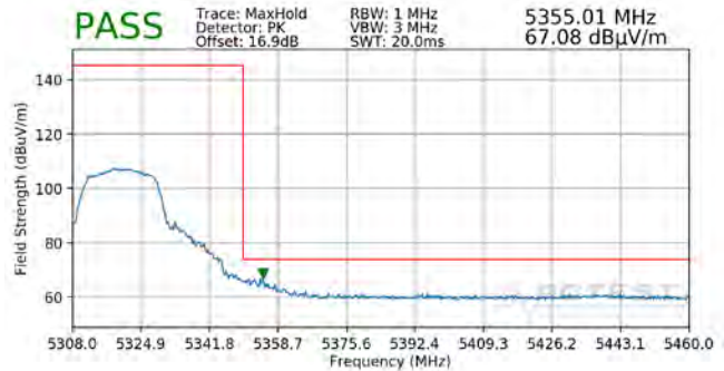
Plot 7-331. Radiated Upper Band Edge Plot SISO ANT2 (Peak – UNII Band 2A)
