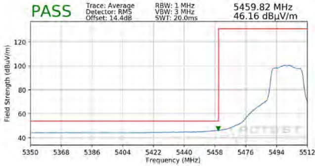
Plot 7-309. Radiated Lower Band Edge Plot SISO ANT1 (Average – UNII Band 2C)
