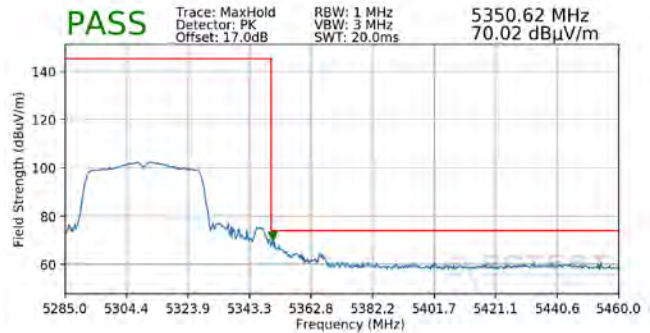
Plot 7-340. Radiated Upper Band Edge Plot SISO ANT2 (Peak – UNII Band 2A)
