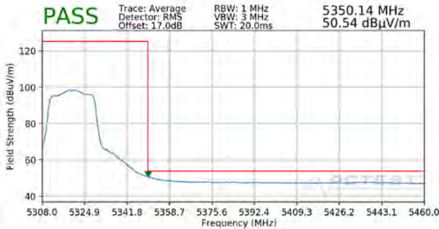
Plot 7-330. Radiated Upper Band Edge Plot SISO ANT2 (Average – UNII Band 2A)
