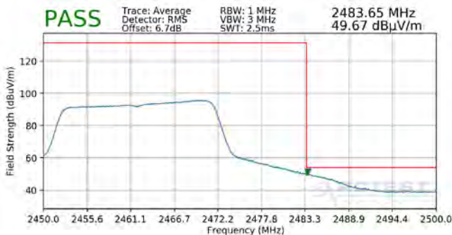
Plot 7-127. Radiated Restricted Upper Band Edge Measurement SISO ANT2 (Average – 242 Tones)
