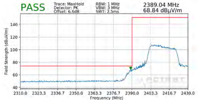
Plot 7-124. Radiated Restricted Lower Band Edge Measurement SISO ANT2 (Peak – 242 Tones)
