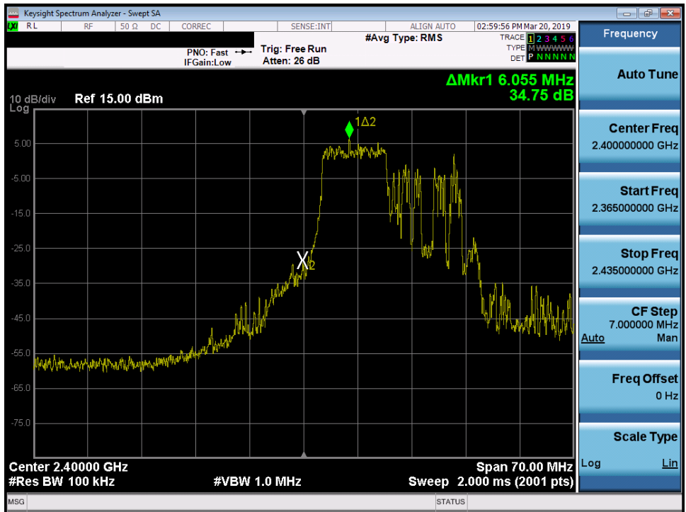
Plot 7-25. Band Edge Plot SISO ANT1 (802.11ax OFDMA – 106 Tones – Ch. 1)
