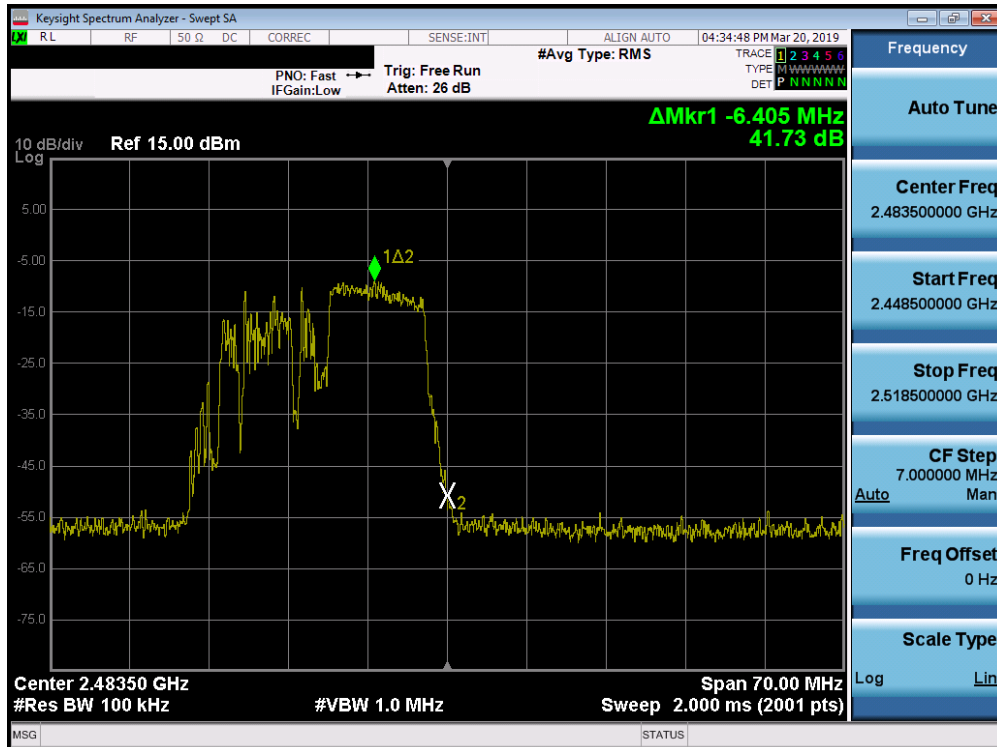
Plot 7-28. Band Edge Plot SISO ANT1 (802.11ax OFDMA – 106 Tones – Ch. 13)
