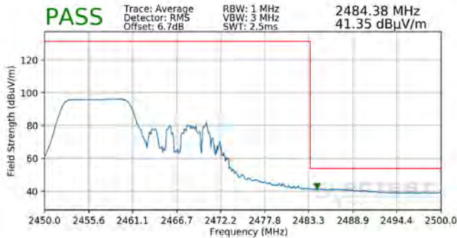
Plot 7-117. Radiated Restricted Upper Band Edge Measurement SISO ANT2 (Average – 106 Tones)
