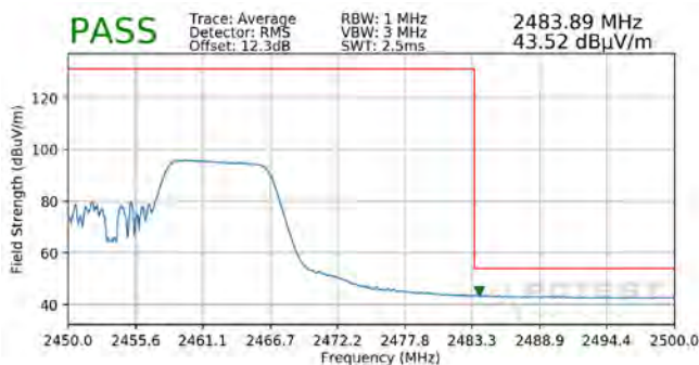
Plot 7-115. Radiated Restricted Upper Band Edge Measurement SISO ANT2 (Average – 106 Tones)
