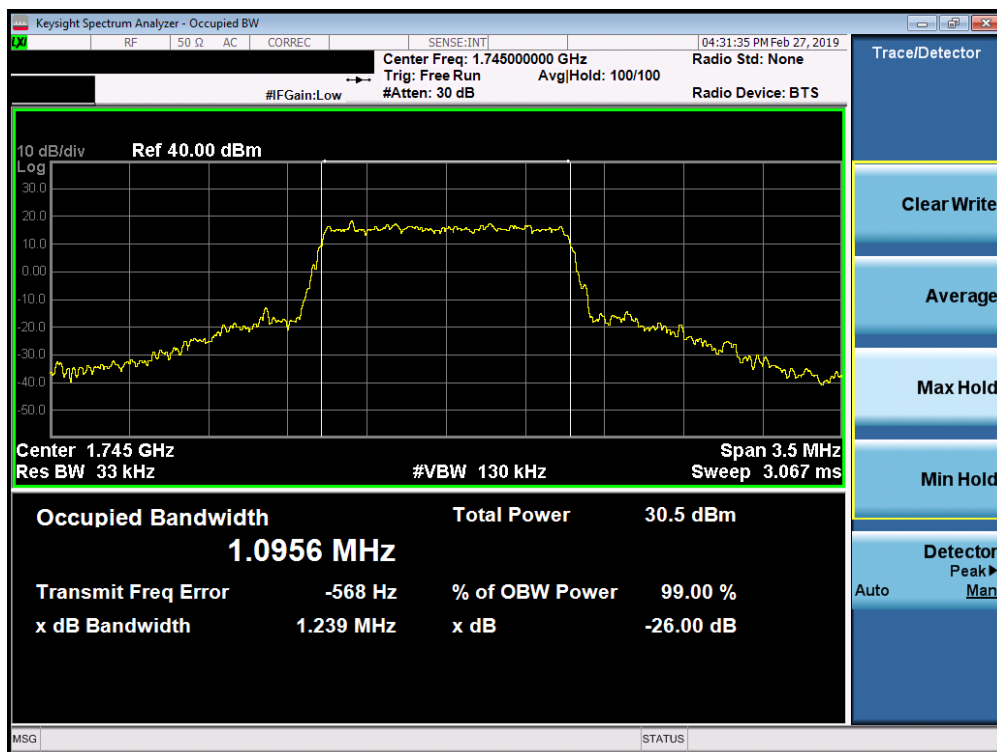
Plot 7-35. Occupied Bandwidth Plot (Band 66/4 - 1.4MHz 16-QAM - Full RB Configuration)
