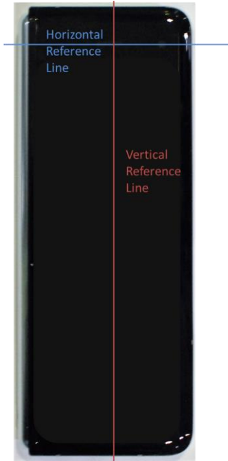
SAR Test Setup Photo 33 – Closed Configuration (Handset) Horizontal and Vertical Reference Lines
