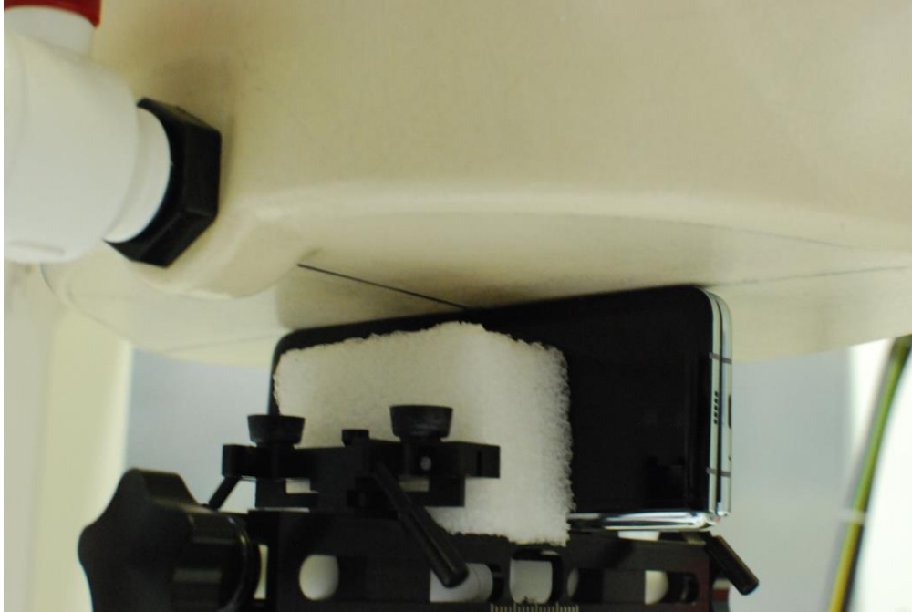
SAR Test Setup Photo 17 – Closed Configuration (Handset) Right Side at 0 mm
