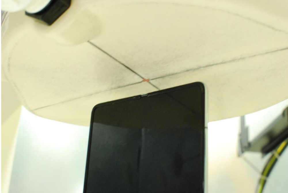
SAR Test Setup Photo 29 – Open Configuration (UMPC) Bottom Side at 10 mm
