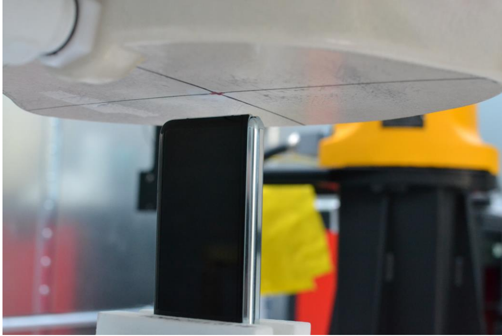
SAR Test Setup Photo 13 – Closed Configuration (Handset) Bottom Side at 13 mm
