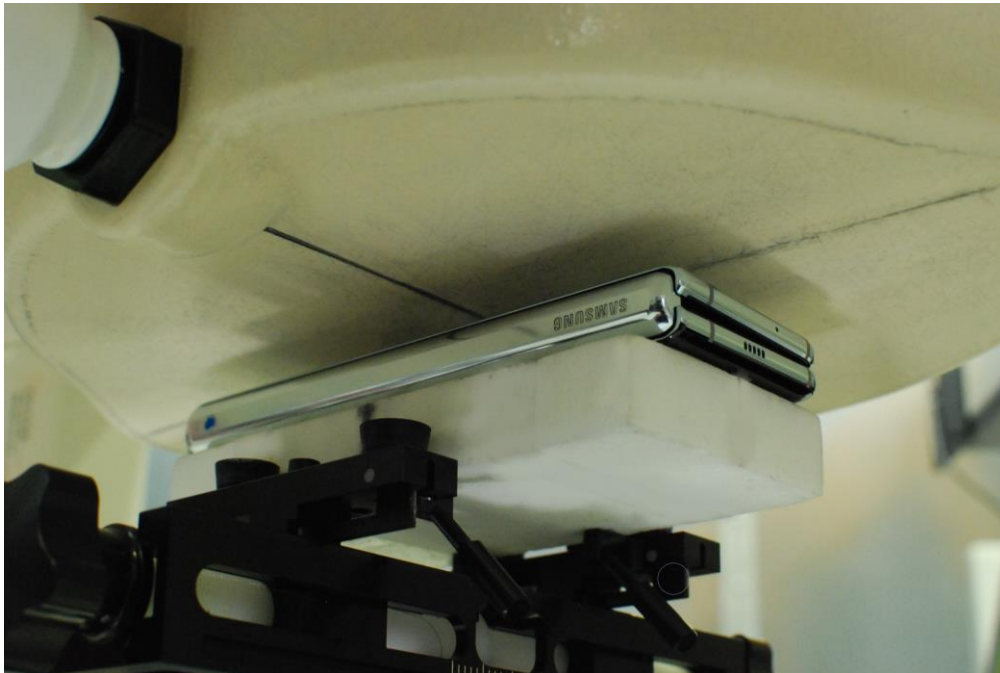
SAR Test Setup Photo 6 – Closed Configuration (Handset) Back Side at 11 mm
