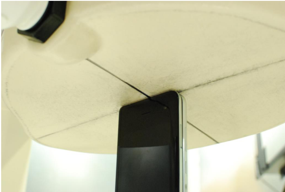
SAR Test Setup Photo 12 – Closed Configuration (Handset) Top Side at 0 mm
