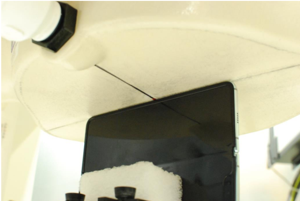
SAR Test Setup Photo 32 – Open Configuration (UMPC) Right Side at 0 mm
