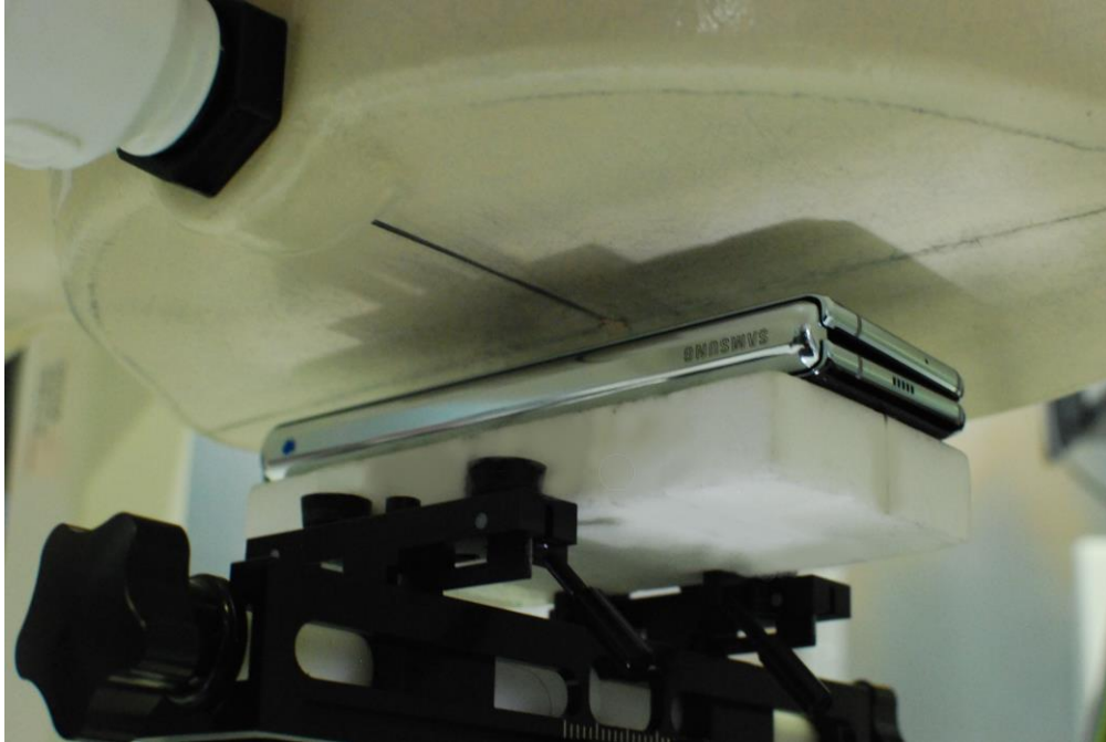
SAR Test Setup Photo 5 – Closed Configuration (Handset) Back Side at 15 mm
