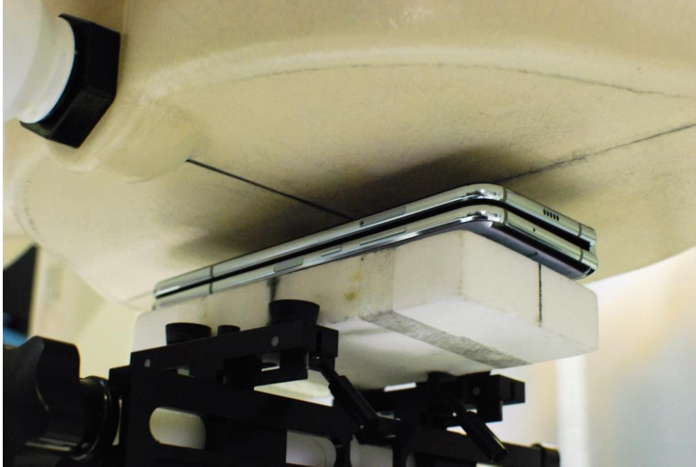
SAR Test Setup Photo 9 – Closed Configuration (Handset) Front Side at 10 mm
