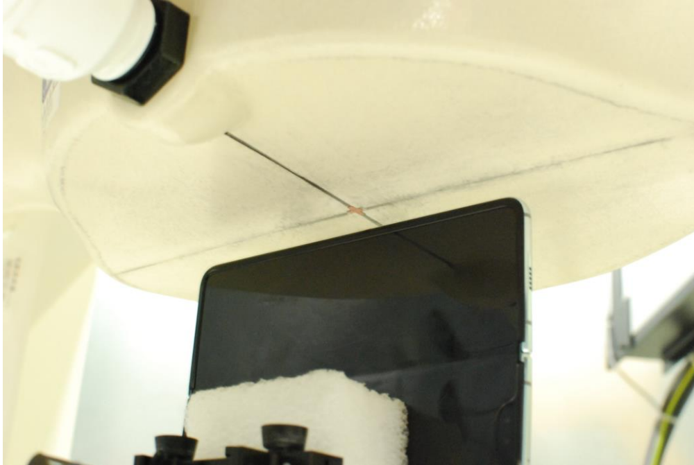
SAR Test Setup Photo 31 – Open Configuration (UMPC) Right Side at 10 mm
