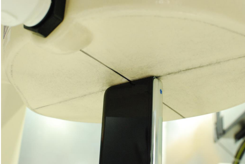
SAR Test Setup Photo 15 – Closed Configuration (Handset) Bottom Side at 0 mm
