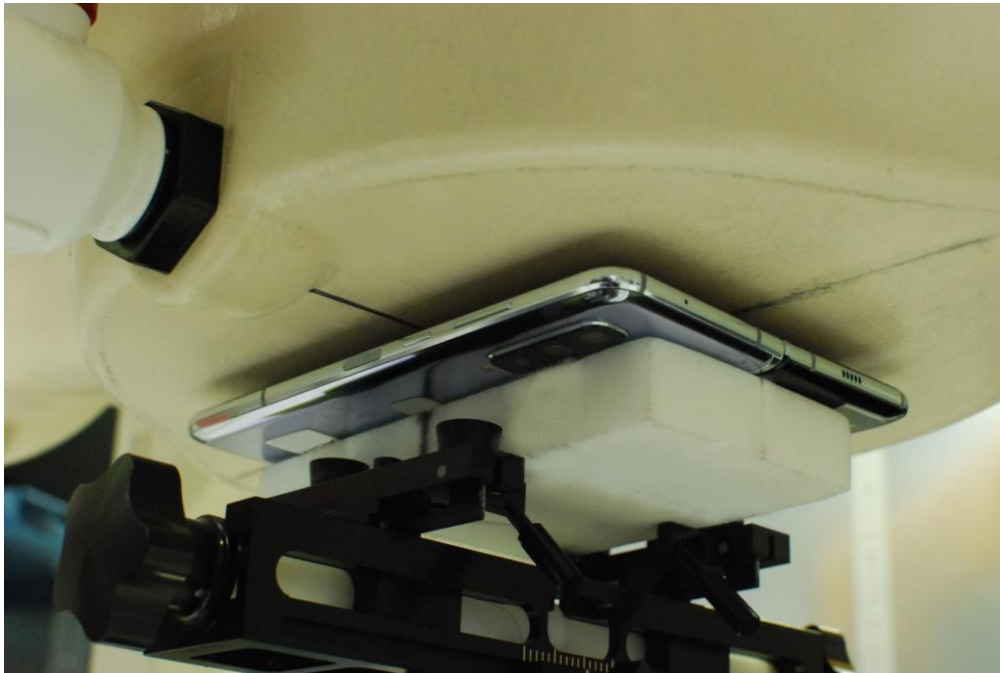
SAR Test Setup Photo 24 – Open Configuration (UMPC) Front Side at 10 mm
