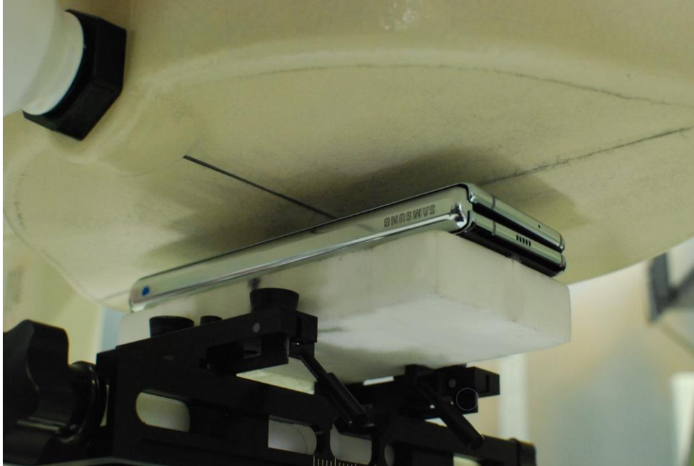
SAR Test Setup Photo 7 – Closed Configuration (Handset) Back Side at 10 mm
