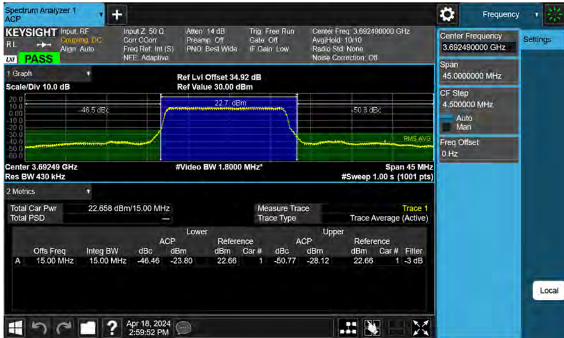
Sub6 n48. Adjacent Channel Leakage Ratio(ACLR) Plot (15 MHz Ch.646166 BPSK RB 36, Offset 0)
