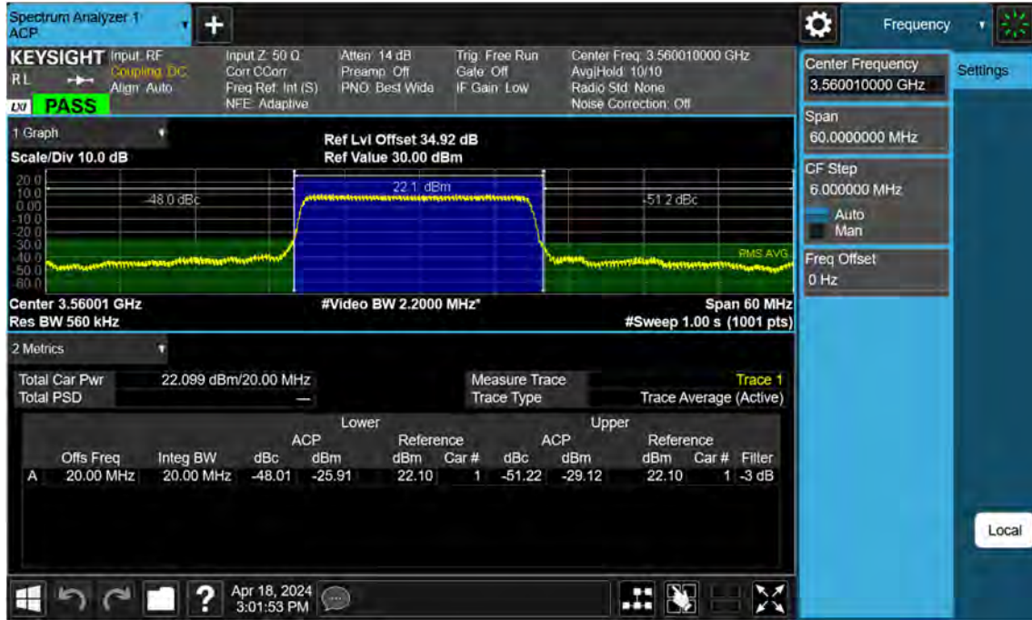
Sub6 n48. Adjacent Channel Leakage Ratio(ACLR) Plot (20 MHz Ch.637334 BPSK RB 50, Offset 0)
