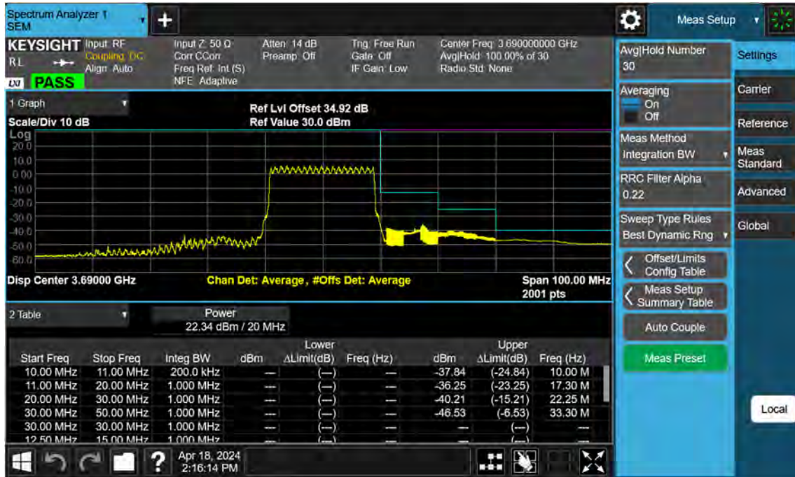
Sub6 n48. 20 M_BandEdge(Upper)_High_ 3690.00 MHz_BPSK_FullRB
