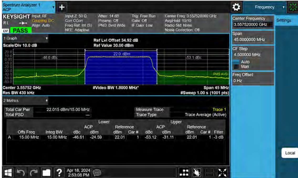
Sub6 n48. Adjacent Channel Leakage Ratio(ACLR) Plot (15 MHz Ch.637168 BPSK RB 36, Offset 0)
