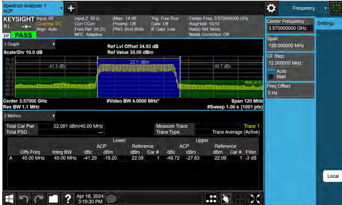
Sub6 n48. Adjacent Channel Leakage Ratio(ACLR) Plot (40 MHz Ch.638000 BPSK RB 100, Offset 0)
