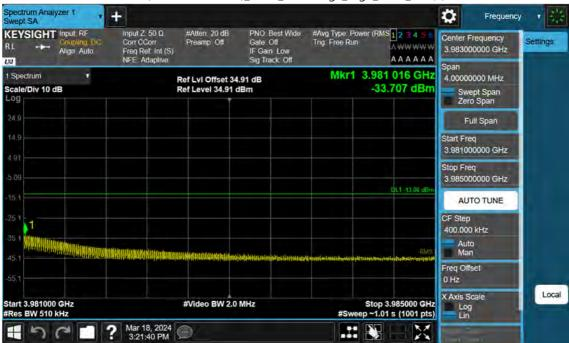
n77(3700~3980 MHz)\_80 M\_Band Edge\_High\_BPSK\_1RB(2)
