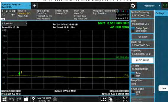
n77(3700~3980 MHz)\_100 M\_Band Edge\_Low\_BPSK\_1RB(3)
