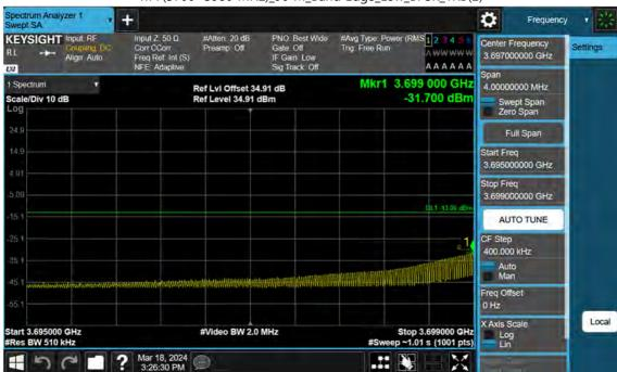
n77(3700~3980 MHz)\_90 M\_Band Edge\_Low\_BPSK\_1RB(2)
