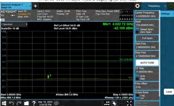
n77(3700~3980 MHz)\_90 M\_Band Edge\_High\_BPSK\_1RB(3)
