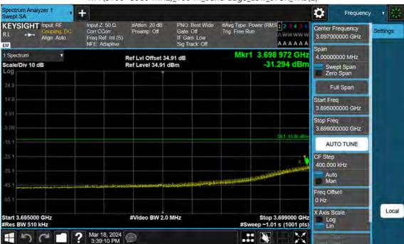
n77(3700~3980 MHz)\_100 M\_Band Edge\_Low\_BPSK\_1RB(2)
