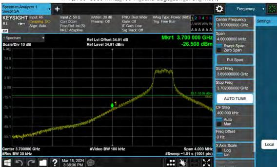
n77(3700~3980 MHz)\_100 M\_Band Edge\_Low\_BPSK\_1RB(1)
