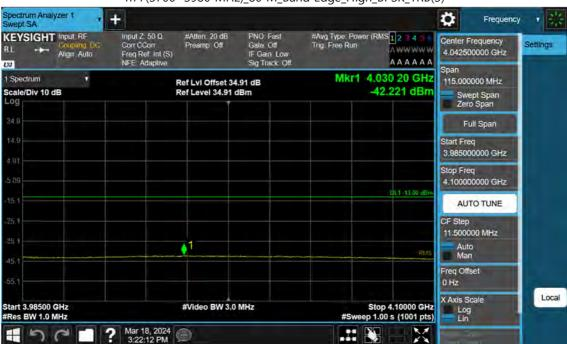
n77(3700~3980 MHz)\_80 M\_Band Edge\_High\_BPSK\_1RB(3)
