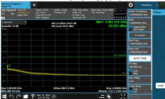
n77(3700~3980 MHz)\_100 M\_Band Edge\_High\_BPSK\_1RB(2)
