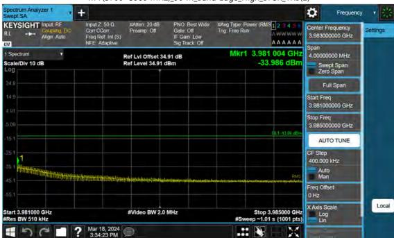
n77(3700~3980 MHz)\_90 M\_Band Edge\_High\_BPSK\_1RB(2)
