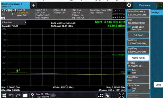
n77(3700~3980 MHz)\_90 M\_Band Edge\_Low\_BPSK\_1RB(3)
