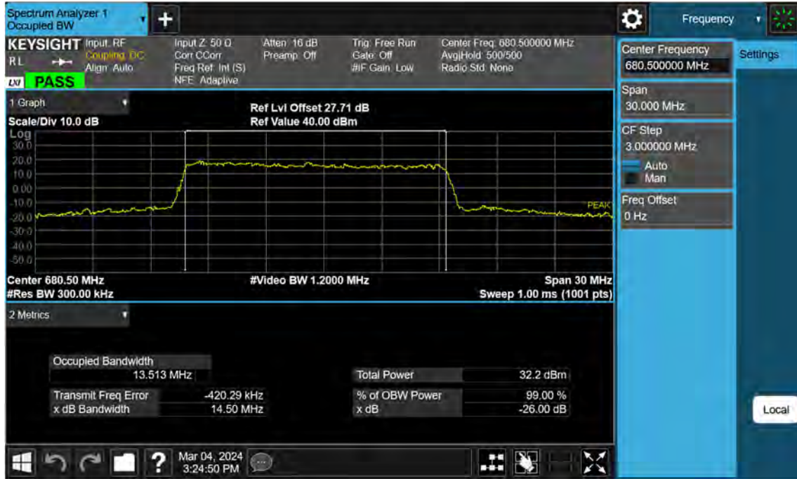
Sub6 n71. Occupied Bandwidth Plot (15 M BW Ch.136100 QPSK_ Full RB)
