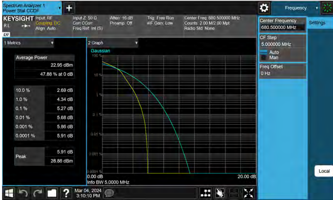
Sub6 n71. PAR Plot (5 M BW_Ch.349000_16QAM_Full RB)
