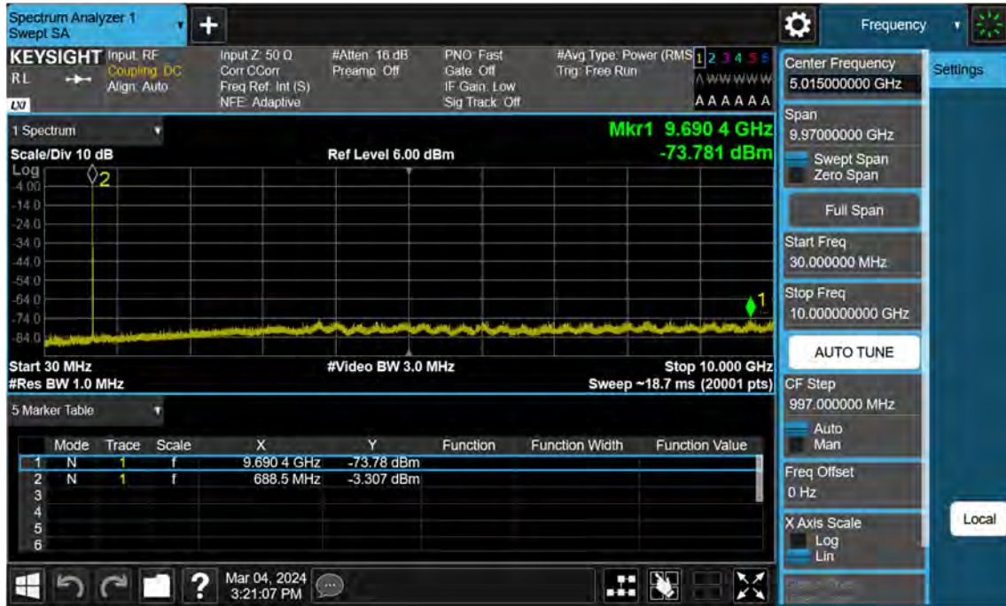
Sub6 n71. Conducted Spurious Plot _ (138600ch_10 MHz_BPSK_RB 1_1)
