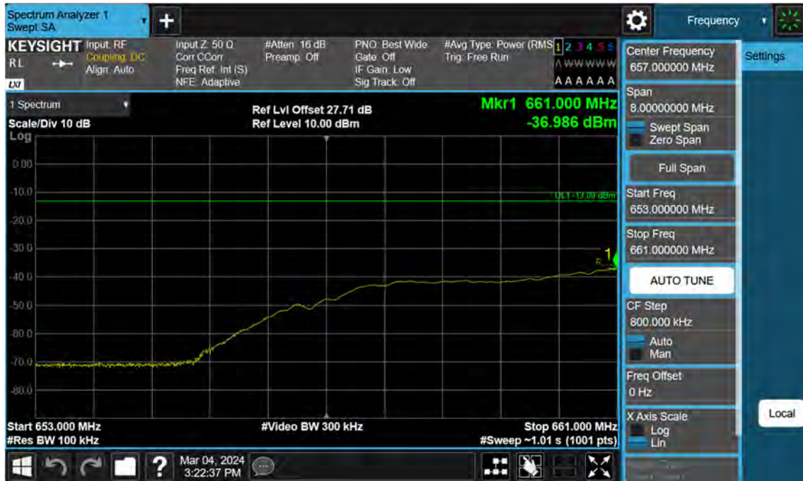
Sub6 n71. Lower Extended Band Edge Plot (15 M BW Ch.134100 BPSK_ Full RB)
