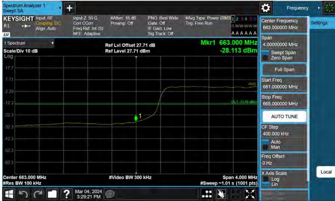
Sub6 n71. Lower Band Edge Plot (20 M BW Ch.134600 BPSK_ Full RB)
