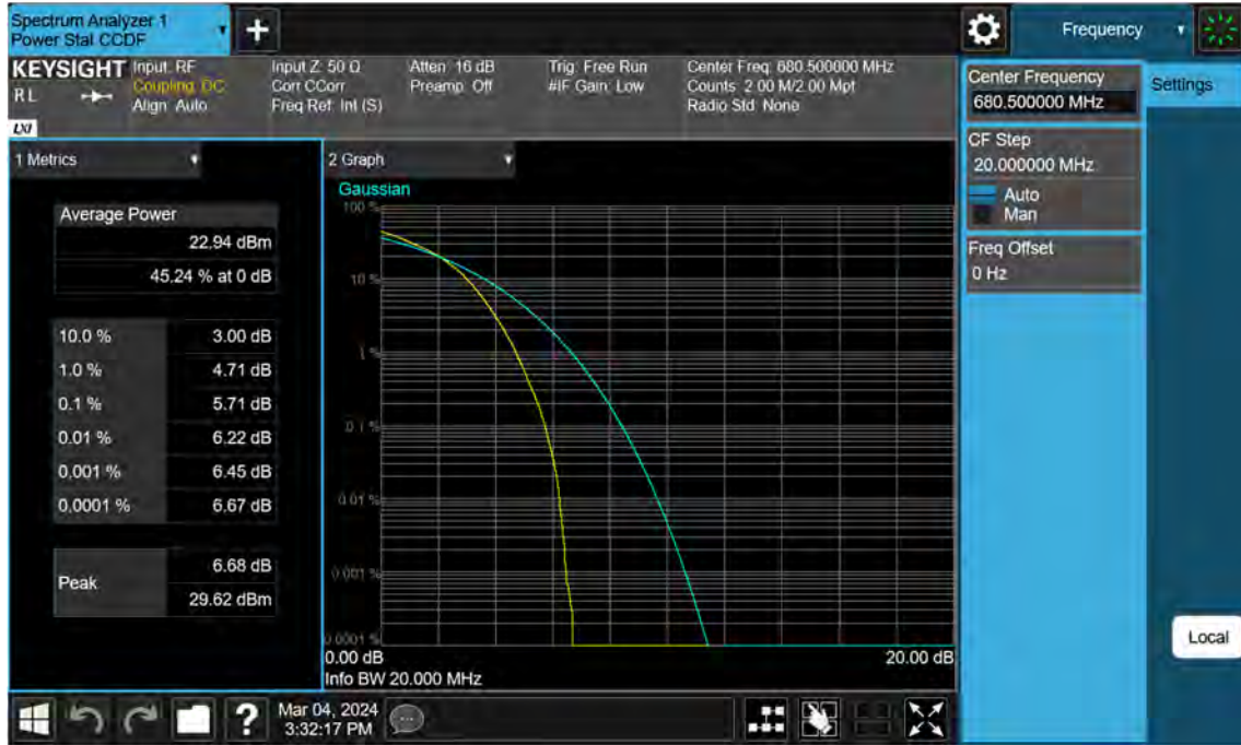
Sub6 n71. PAR Plot (20 M BW_Ch.349000_16QAM_Full RB)
