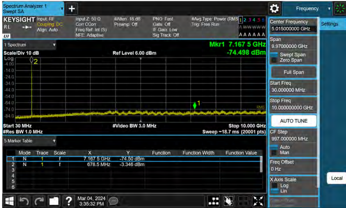
Sub6 n71. Conducted Spurious Plot _ (137600ch_20 MHz_BPSK_RB 1_1)
