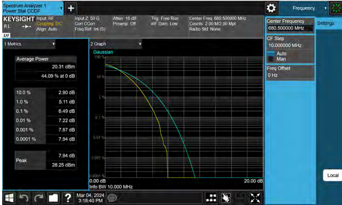
Sub6 n71. PAR Plot (10 M BW_Ch.349000_256QAM_Full RB)
