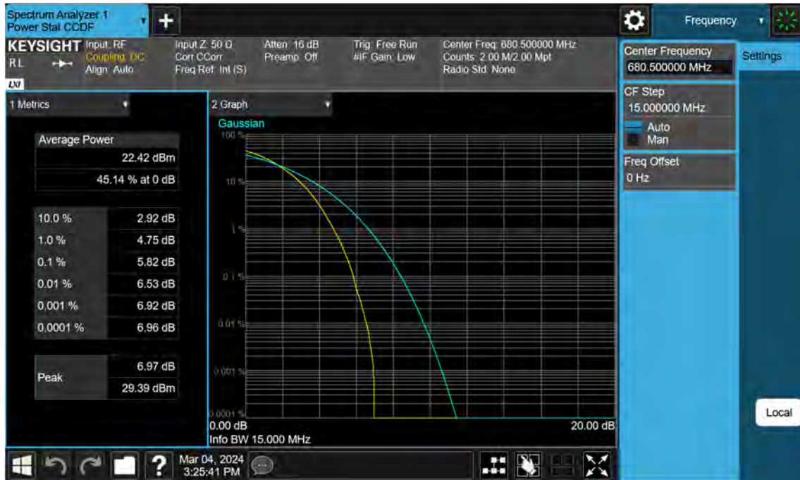
Sub6 n71. PAR Plot (15 M BW_Ch.349000_64QAM_Full RB)
