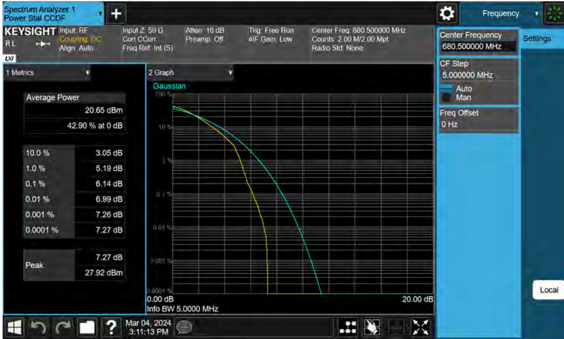
Sub6 n71. PAR Plot (5 M BW_Ch.349000_256QAM_Full RB)
