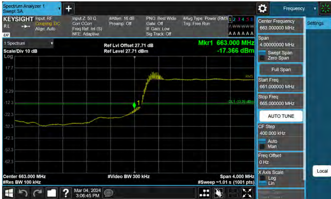
Sub6 n71. Lower Band Edge Plot (5 M BW Ch.133100 BPSK_ Full RB)
