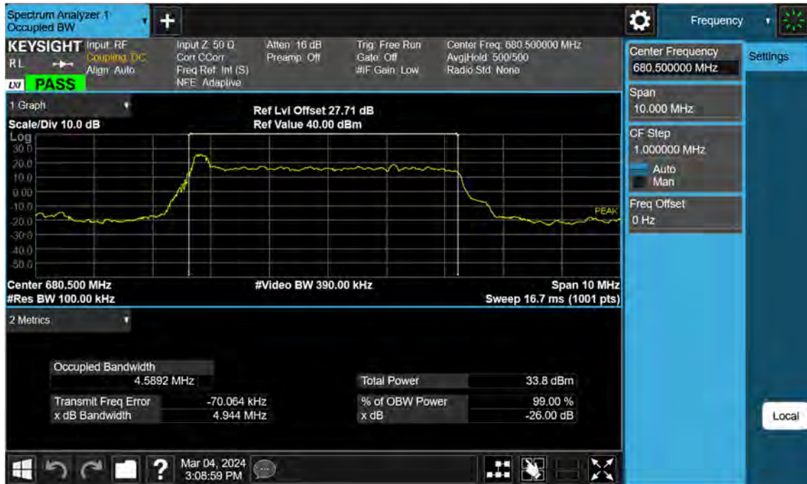
Sub6 n71. Occupied Bandwidth Plot (5 M BW Ch.136100 BPSK_Full RB)
