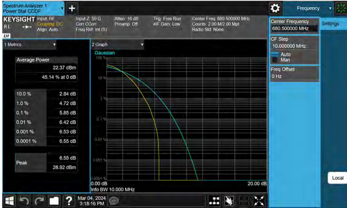
Sub6 n71. PAR Plot (10 M BW_Ch.349000_64QAM_Full RB)
