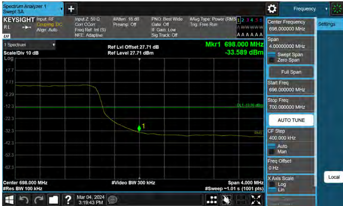
Sub6 n71. Upper Band Edge Plot (10 M BW Ch.138600 BPSK_ Full RB)
