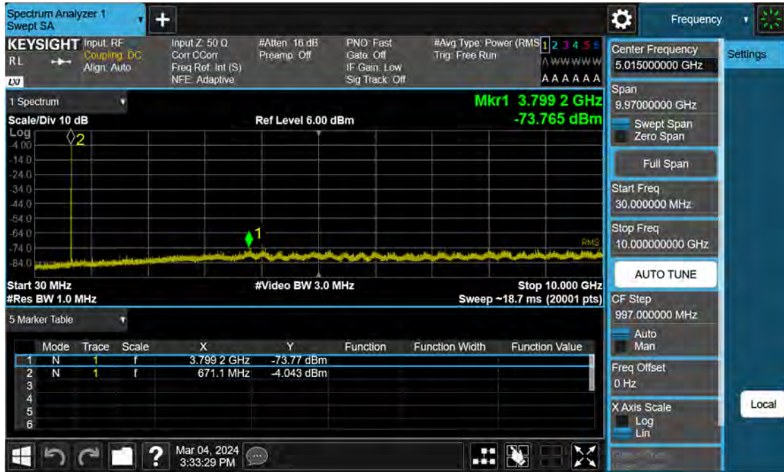
Sub6 n71. Conducted Spurious Plot _ (136100ch_20 MHz_BPSK_RB 1_1)
