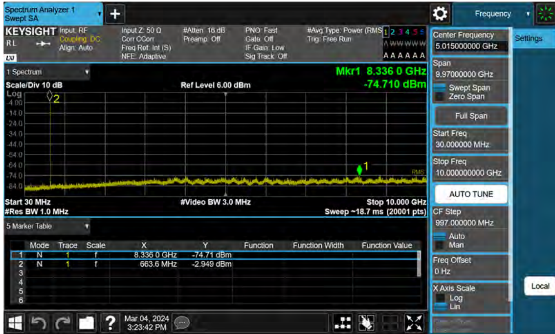
Sub6 n71. Conducted Spurious Plot _ (134100ch_15 MHz_BPSK_RB 1_1)
