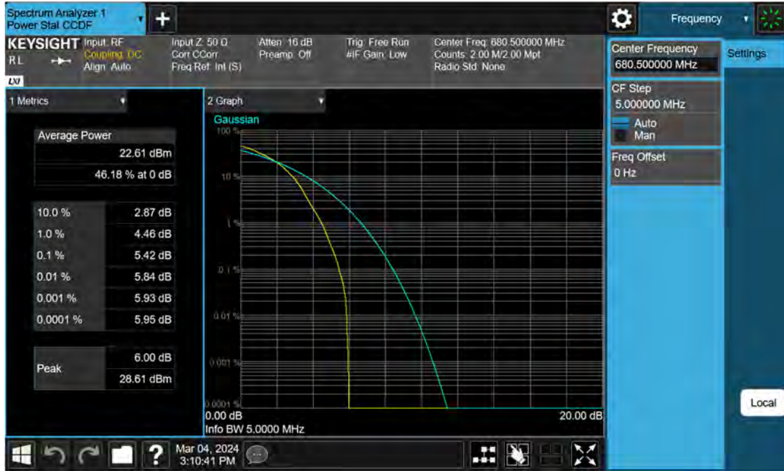
Sub6 n71. PAR Plot (5 M BW_Ch.349000_64QAM_Full RB)
