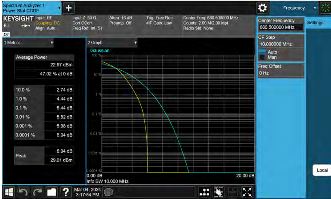
Sub6 n71. PAR Plot (10 M BW_Ch.349000_16QAM_Full RB)
