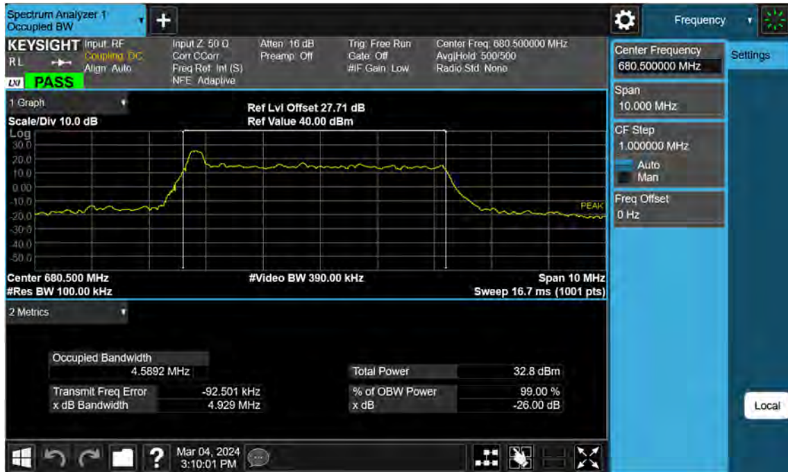
Sub6 n71. Occupied Bandwidth Plot (5 M BW Ch.136100 16QAM_ Full RB)
