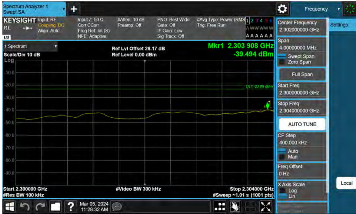
NR30_10 M_Band Edge(2300MHz-2304MHz)_Mid_BPSK_FullRB
