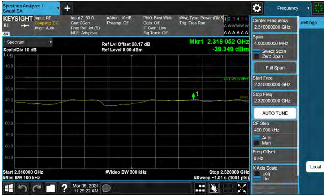
NR30_10 M_Band Edge(2316MHz-2320MHz)_Mid_BPSK_FullRB
