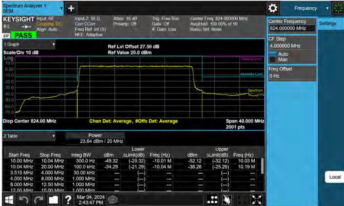
Sub6 n26. Mid Channel Edge Plot (20 M BW Ch.164800 BPSK_ RB100_Offset 0)
