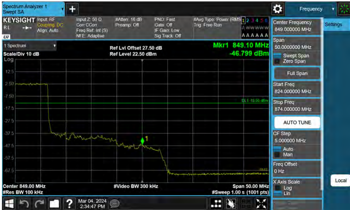
Sub6 n26. Upper Band Edge Plot (15 M BW Ch.164800 BPSK_RB75_Offset 0)
