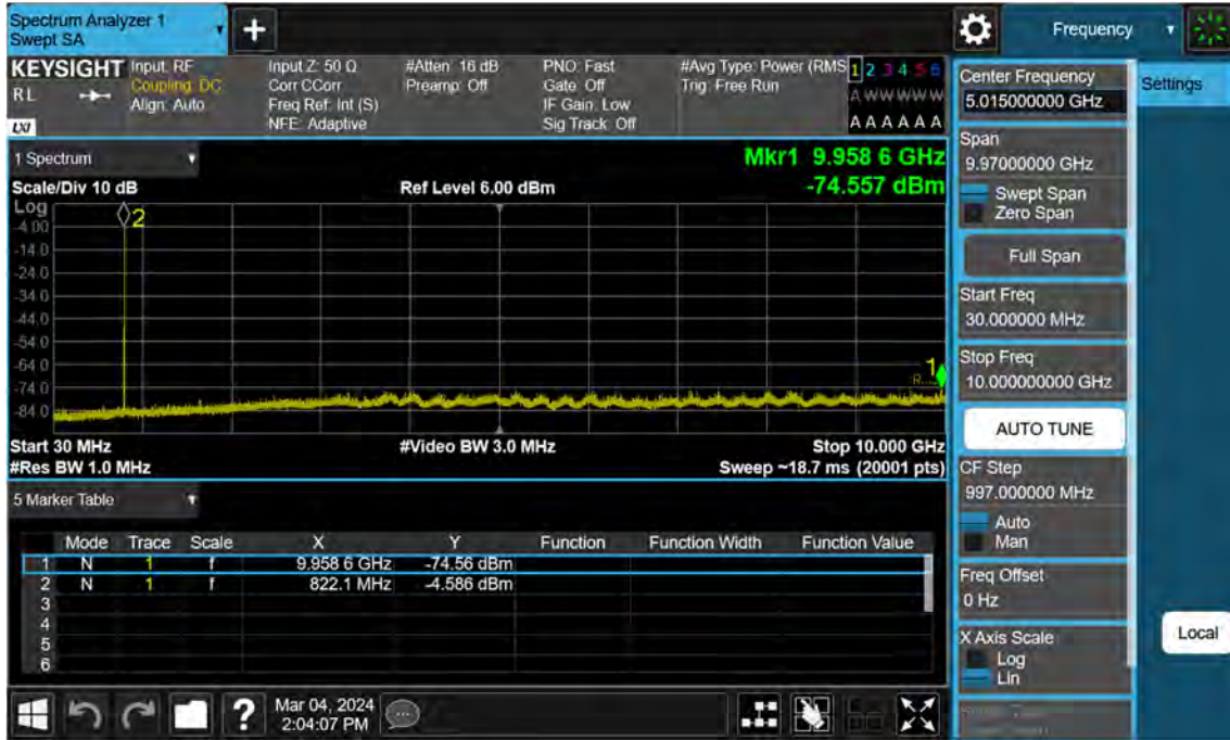
Sub6 n26. Conducted Spurious (164800 ch_5 MHz_ BPSK_RB 1_1)
