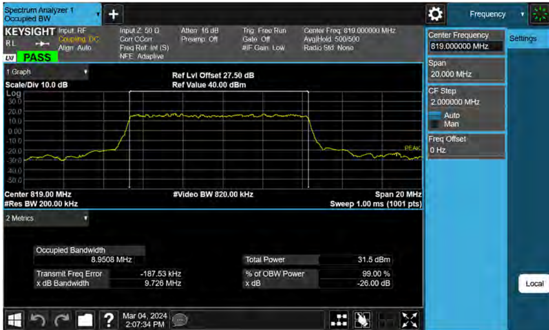
Sub6 n26. Occupied Bandwidth Plot (10 M BW Ch.163800 BPSK RB 50_0)
