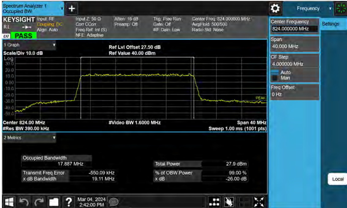
Sub6 n26. Occupied Bandwidth Plot (20 M BW Ch.164800 256QAM RB 100_0)
