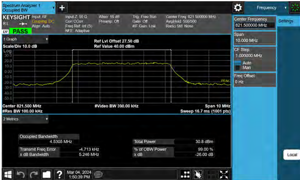
Sub6 n26. Occupied Bandwidth Plot (5 M BW Ch.164300 QPSK RB 25_0)
