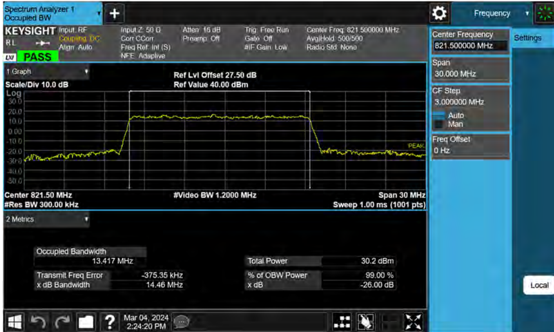
Sub6 n26. Occupied Bandwidth Plot (15 M BW Ch.164300 16QAM RB 75_0)
