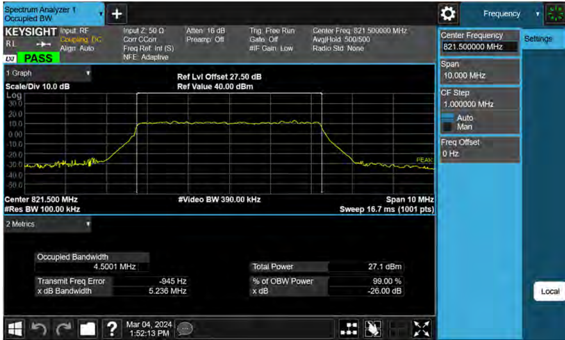
Sub6 n26. Occupied Bandwidth Plot (5 M BW Ch.164300 256QAM RB 25_0)
