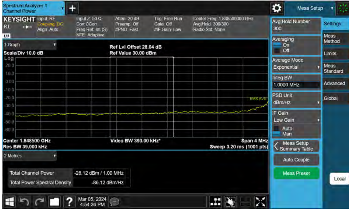
Sub6 n25(2)_35 M_Extended Band Edge_Low_BPSK_FullRB
