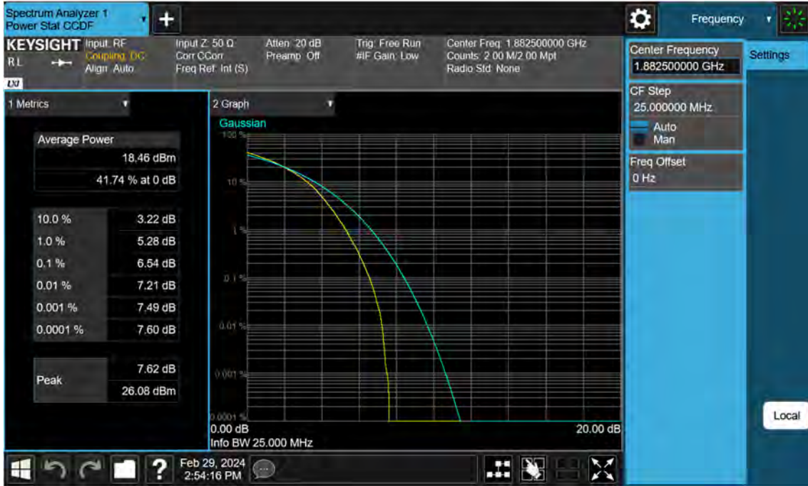
Sub6 n25_25 M_PAR_Mid_256QAM_FullRB
