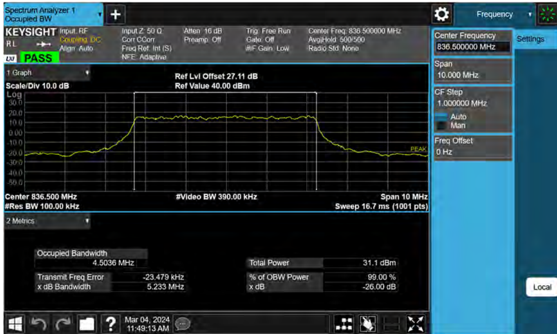
Sub6 n5. Occupied Bandwidth Plot (5 M BW Ch.167300 BPSK_Full RB_0)
