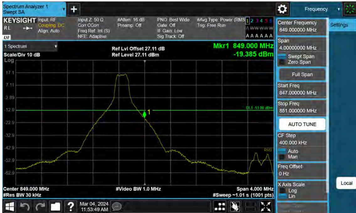
Sub6 n5. Upper Band Edge Plot (5 M BW Ch.169300 BPSK_RB1_Offset 24)
