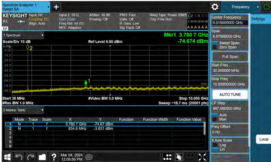
Sub6 n5. Conducted Spurious Plot (168300ch_15 MHz_BPSK_RB 1_1)
