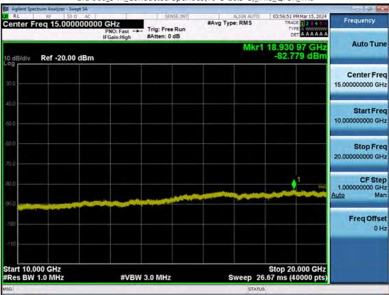
LTE B66\_3 M\_Conducted Spurious(10 G-26.5 G)\_Mid\_QPSK\_1RB
