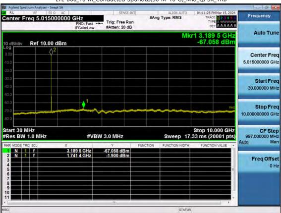
LTE B66\_10 M\_Conducted Spurious(30 M-10 G)\_Mid\_QPSK\_1RB
