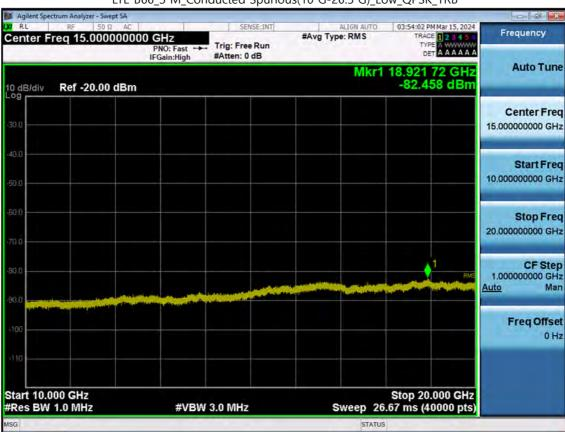
LTE B66\_3 M\_Conducted Spurious(10 G-26.5 G)\_Low\_QPSK\_1RB
