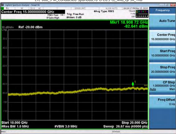
LTE B66\_5 M\_Conducted Spurious(10 G-26.5 G)\_Mid\_QPSK\_1RB
