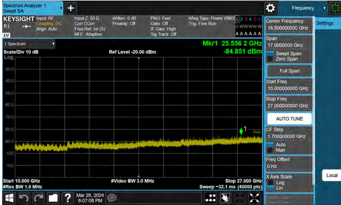
Sub6 n41_50 M_Conducted Spurious(Above10 G)_High_BPSK_1RB
