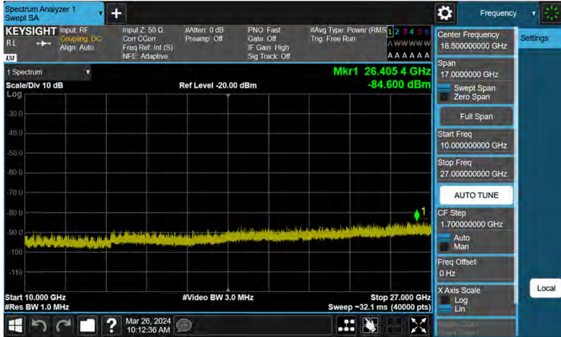
Sub6 n38_30 M_Conducted Spurious(Above10 G)_High_BPSK_1RB
