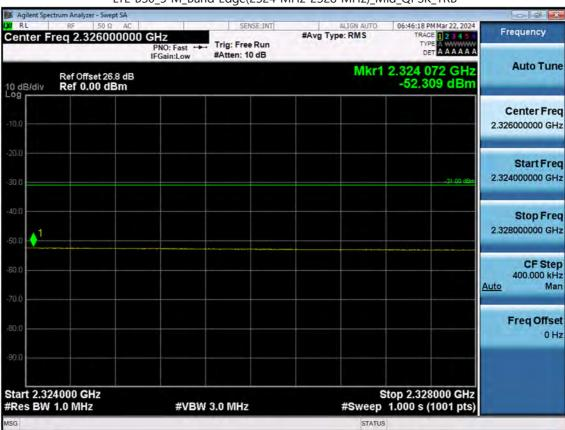
LTE B30\_5 M\_Band Edge(2324 MHz-2328 MHz)\_Mid\_QPSK\_1RB
