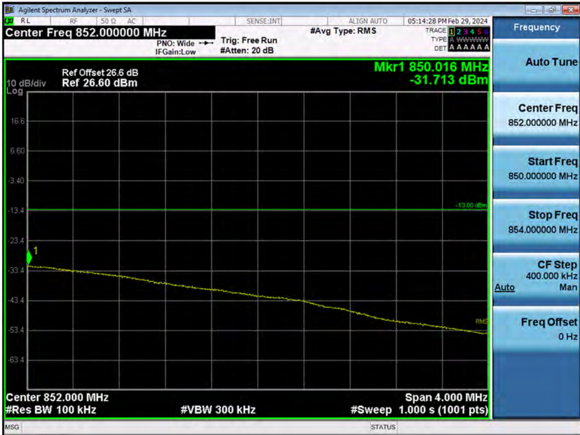
BAND5/26. Upper Extended Band Edge Plot (3 M BW Ch.27025 QPSK_RB15_0)
