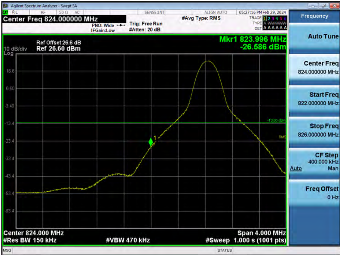
BAND 26. Lower Band Edge Plot (15 M BW Ch.26865 QPSK_RB1_Offset 0)
