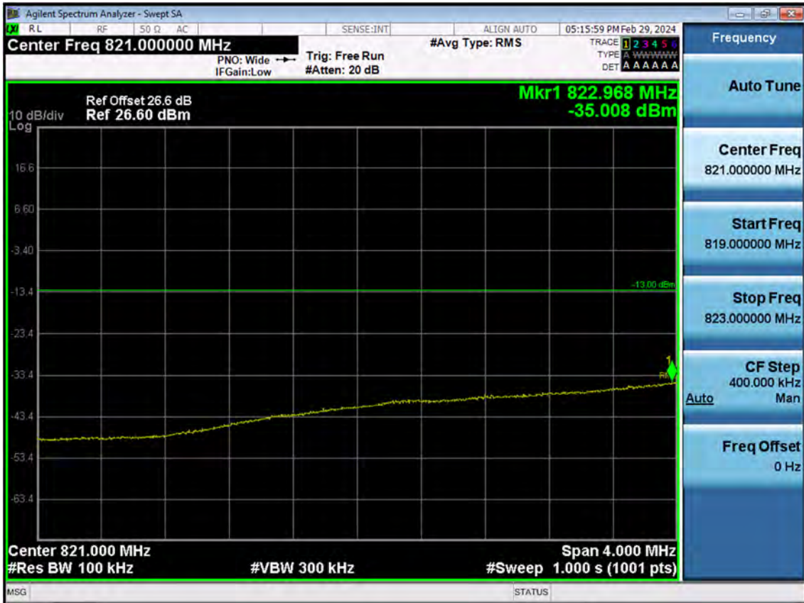
BAND5/26. Lower Extended Band Edge Plot (5 M BW Ch.26815 QPSK_RB25_0)
