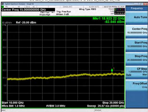
LTE B25\_3 M\_Conducted Spurious(10 G-26.5 G)\_Low\_QPSK\_1RB
