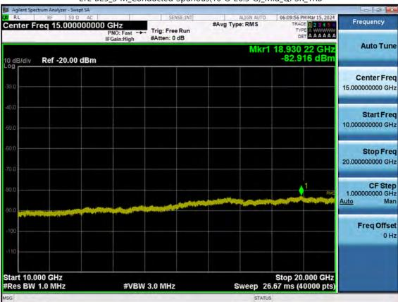
LTE B25\_3 M\_Conducted Spurious(10 G-26.5 G)\_Mid\_QPSK\_1RB
