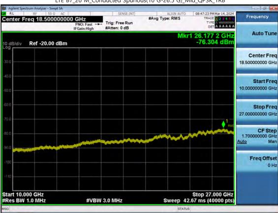
LTE B7\_20 M\_Conducted Spurious(10 G-26.5 G)\_Mid\_QPSK\_1RB
