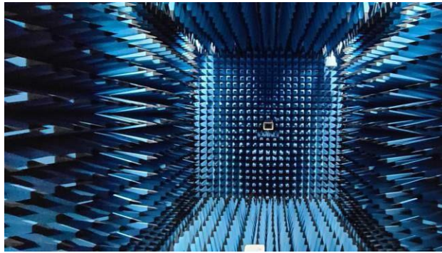
Figure 2: Geometry of Anechoic Chamber for Radiation patterns.
