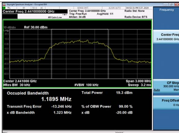
Dual ANT. 1 8DPSK 20 dB BW &amp; 99% OBW (CH. 39)
