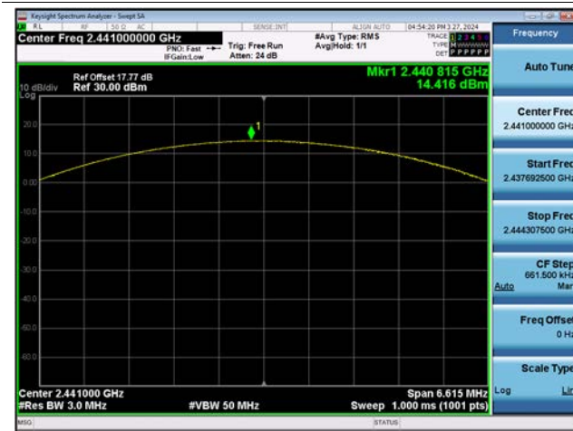
Dual ANT.1 \pi /4DQPSK : Peak Power (CH. 39)
