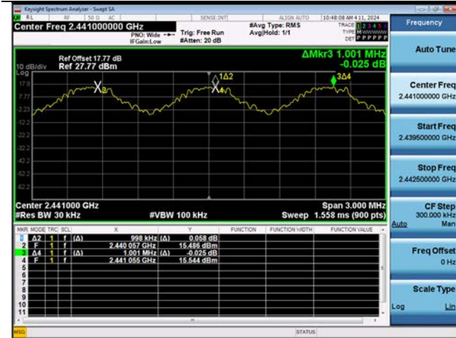
ANT. 1 \pi /4DQPSK : Channel Separation
