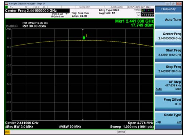
ANT.2 8DPSK : Peak Power (CH. 39)
