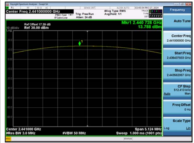
Dual ANT.2 8DPSK : Peak Power (CH. 39)
