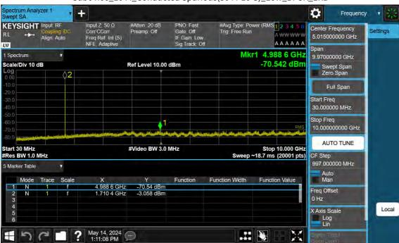
Sub6 n66\_10 M\_Conducted Spurious(30 M-10 G)\_Low\_BPSK\_1RB
