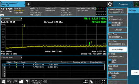
Sub6 n66\_35 M\_Conducted Spurious(30 M-10 G)\_Low\_BPSK\_1RB
