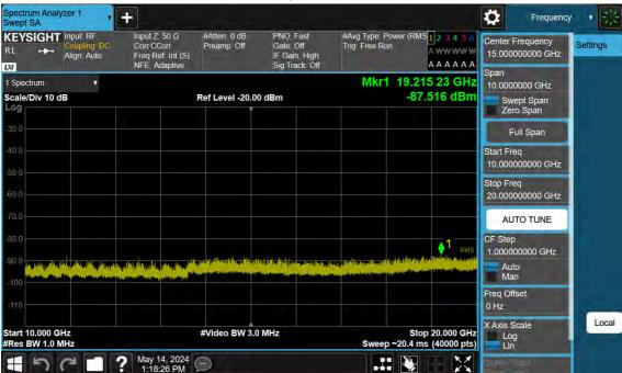
Sub6 n66\_15 M\_Conducted Spurious(Above10 G)\_Low\_BPSK\_1RB
