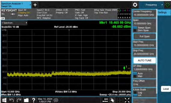
Sub6 n66\_35 M\_Conducted Spurious(Above10 G)\_Low\_BPSK\_1RB
