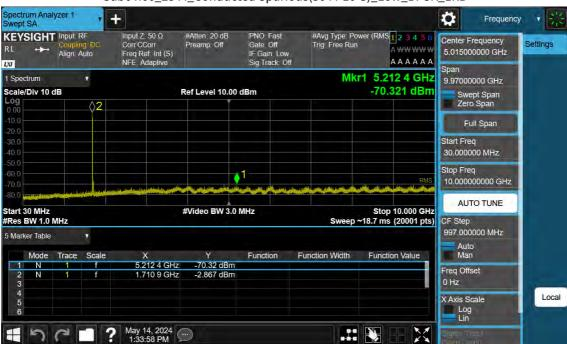
Sub6 n66\_25 M\_Conducted Spurious(30 M-10 G)\_Low\_BPSK\_1RB
