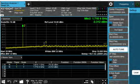
Sub6 n66\_20 M\_Conducted Spurious(30 M-10 G)\_Low\_BPSK\_1RB
