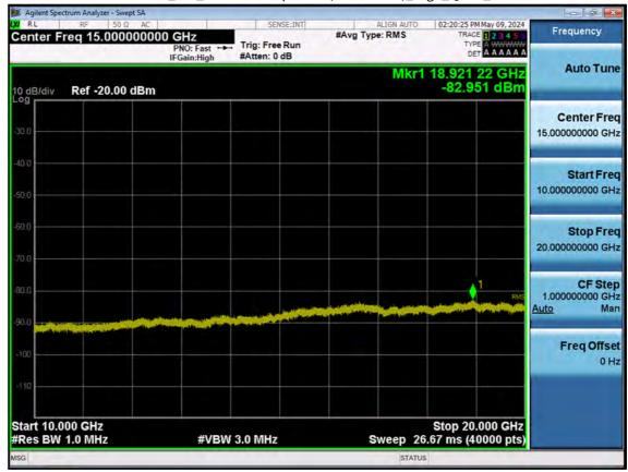
LTE B66\_3 M\_Conducted Spurious(10 G-26.5 G)\_High\_QPSK\_1RB
