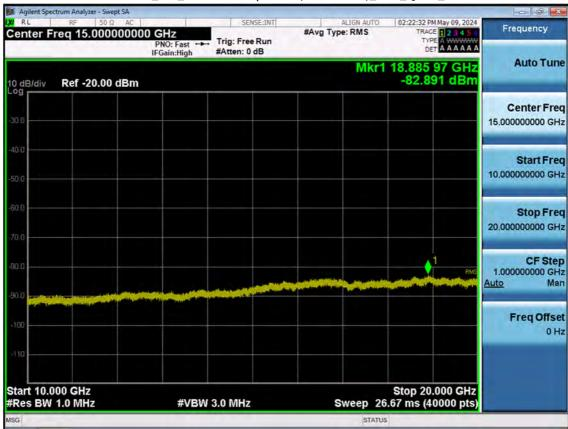
LTE B66\_5 M\_Conducted Spurious(10 G-26.5 G)\_Low\_QPSK\_1RB
