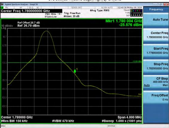
LTE B66\_15 M\_Band Edge\_High\_QPSK\_1RB
