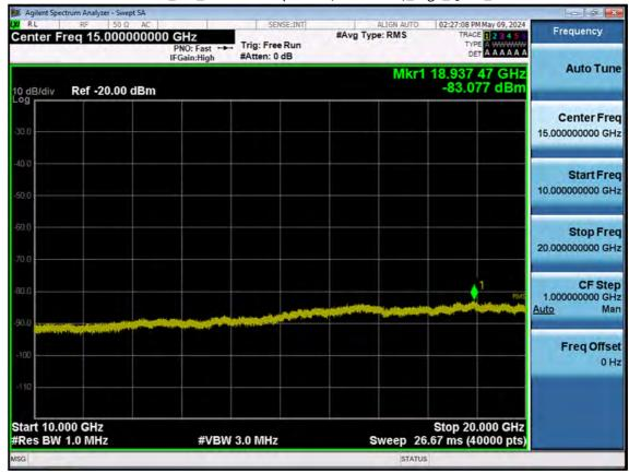
LTE B66\_5 M\_Conducted Spurious(10 G-26.5 G)\_High\_QPSK\_1RB
