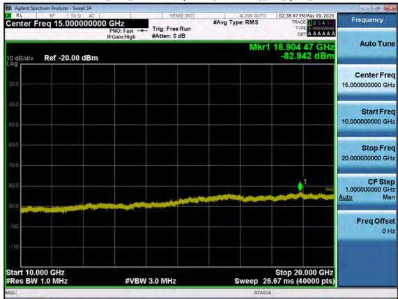
LTE B66\_15 M\_Conducted Spurious(10 G-26.5 G)\_Mid\_QPSK\_1RB
