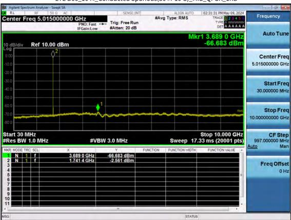
LTE B66\_10 M\_Conducted Spurious(30 M-10 G)\_Mid\_QPSK\_1RB
