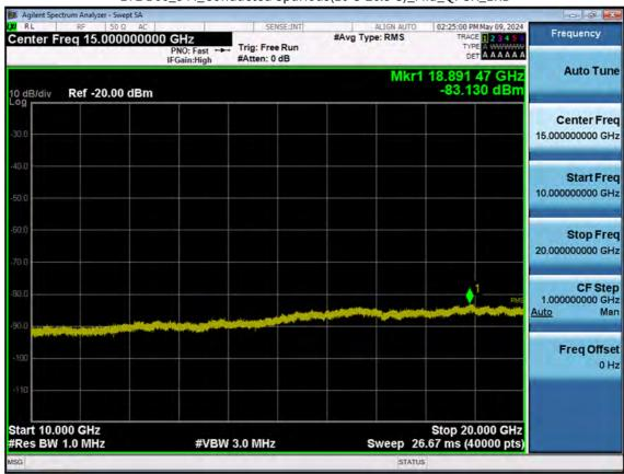
LTE B66\_5 M\_Conducted Spurious(10 G-26.5 G)\_Mid\_QPSK\_1RB
