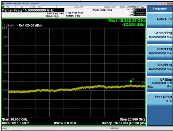
LTE B66\_1.4 M\_Conducted Spurious(10 G-26.5 G)\_Mid\_QPSK\_1RB
