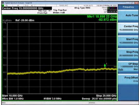
LTE B66\_15 M\_Conducted Spurious(10 G-26.5 G)\_Low\_QPSK\_1RB
