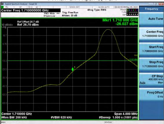
LTE B66\_20 M\_Band Edge\_Low\_QPSK\_1RB
