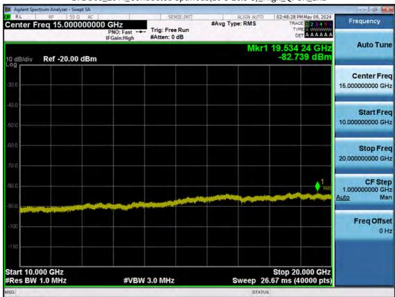
LTE B66\_20 M\_Conducted Spurious(10 G-26.5 G)\_High\_QPSK\_1RB
