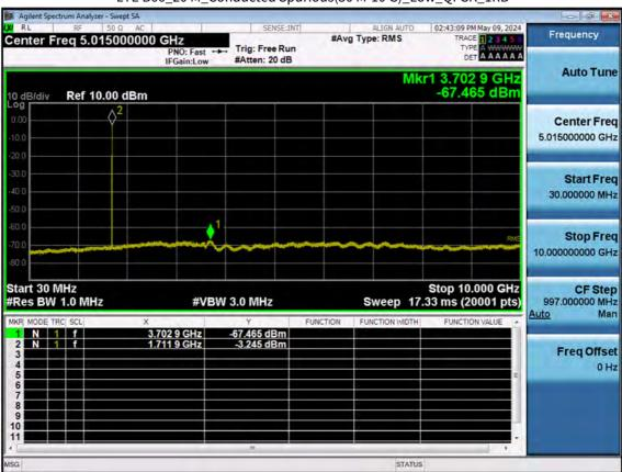
LTE B66\_20 M\_Conducted Spurious(30 M-10 G)\_Low\_QPSK\_1RB
