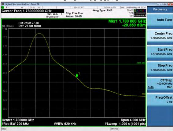
LTE B66\_20 M\_Band Edge\_High\_QPSK\_1RB
