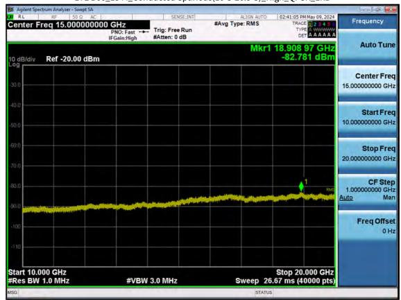
LTE B66\_15 M\_Conducted Spurious(10 G-26.5 G)\_High\_QPSK\_1RB
