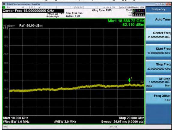
LTE B66\_20 M\_Conducted Spurious(10 G-26.5 G)\_Low\_QPSK\_1RB
