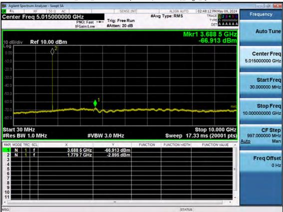
LTE B66\_20 M\_Conducted Spurious(30 M-10 G)\_High\_QPSK\_1RB
