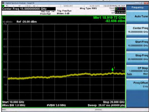
LTE B66\_10 M\_Conducted Spurious(10 G-26.5 G)\_High\_QPSK\_1RB
