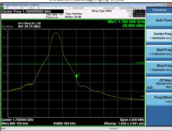
LTE B66\_10 M\_Band Edge\_High\_QPSK\_1RB
