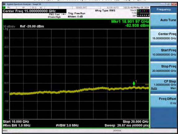
LTE B66\_10 M\_Conducted Spurious(10 G-26.5 G)\_Mid\_QPSK\_1RB
