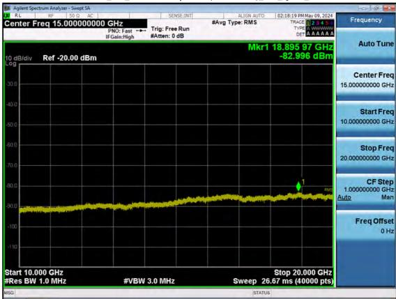
LTE B66\_3 M\_Conducted Spurious(10 G-26.5 G)\_Mid\_QPSK\_1RB
