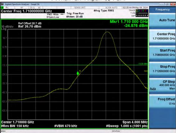
LTE B66\_15 M\_Band Edge\_Low\_QPSK\_1RB
