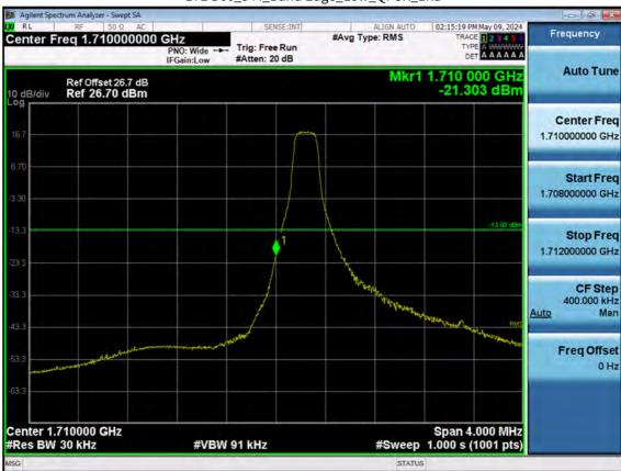
LTE B66\_3 M\_Band Edge\_Low\_QPSK\_1RB
