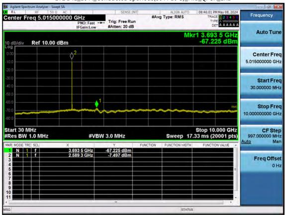
LTE B41\_10 M\_Conducted Spurious(30 M-10 G)\_Mid\_QPSK\_1RB
