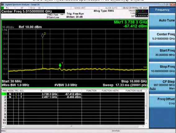
LTE B41\_10 M\_Conducted Spurious(30 M-10 G)\_Low\_QPSK\_1RB
