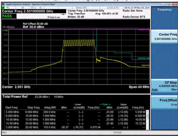
LTE B41\_10 M\_Channel Edge\_Upper\_Low\_QPSK\_FullRB
