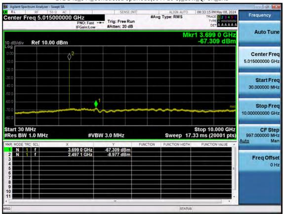
LTE B41\_5 M\_Conducted Spurious(30 M-10 G)\_Low\_QPSK\_1RB
