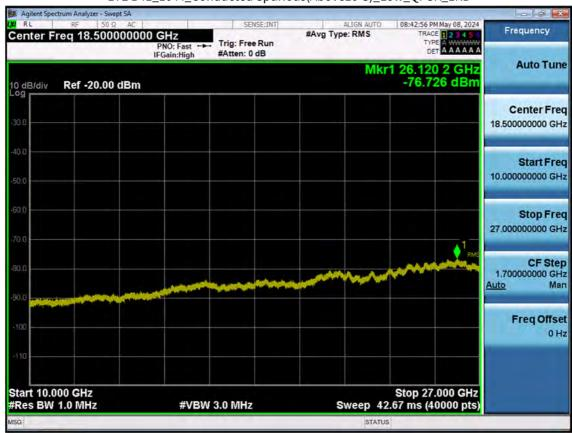
LTE B41\_10 M\_Conducted Spurious(Above10 G)\_Low\_QPSK\_1RB
