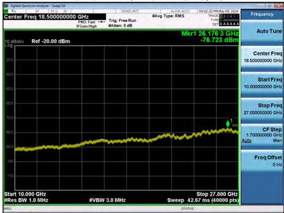
LTE B41\_20 M\_Conducted Spurious(Above10 G)\_Low\_QPSK\_1RB
