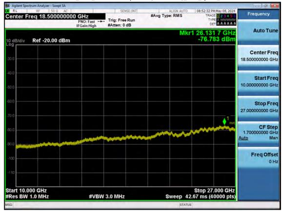
LTE B41\_15 M\_Conducted Spurious(Above10 G)\_Low\_QPSK\_1RB
