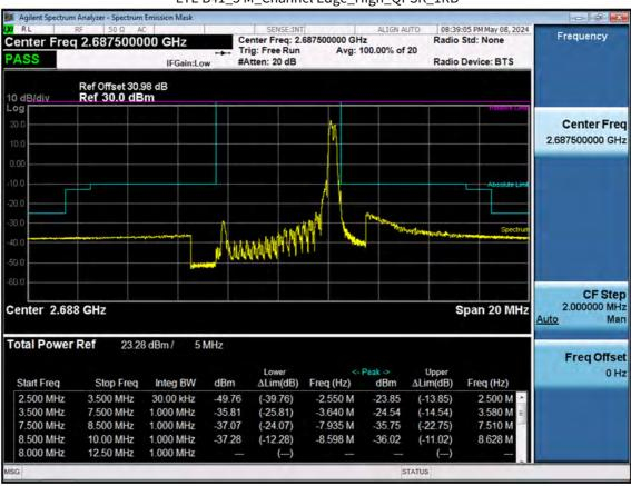
LTE B41\_5 M\_Channel Edge\_High\_QPSK\_1RB
