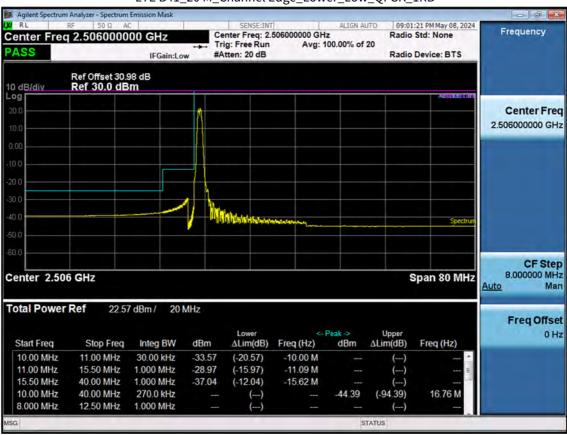
LTE B41\_20 M\_Channel Edge\_Lower\_Low\_QPSK\_1RB
