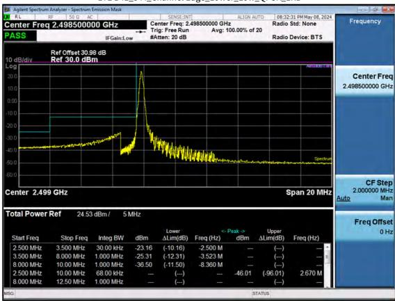
LTE B41\_5 M\_Channel Edge\_Lower\_Low\_QPSK\_1RB
