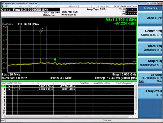
LTE B41\_20 M\_Conducted Spurious(30 M-10 G)\_Mid\_QPSK\_1RB
