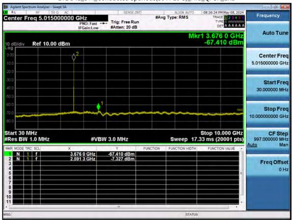
LTE B41\_5 M\_Conducted Spurious(30 M-10 G)\_Mid\_QPSK\_1RB
