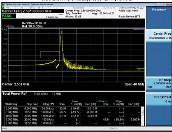
LTE B41\_10 M\_Channel Edge\_Lower\_Low\_QPSK\_1RB
