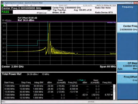
LTE B41\_15 M\_Channel Edge\_Lower\_Low\_QPSK\_1RB
