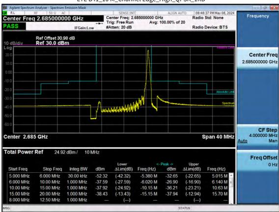
LTE B41\_10 M\_Channel Edge\_High\_QPSK\_1RB
