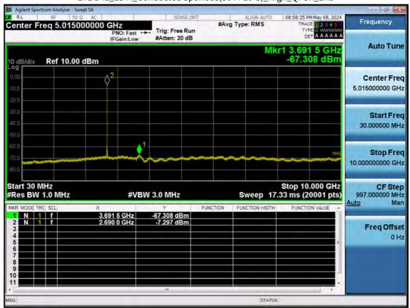
LTE B41\_15 M\_Conducted Spurious(30 M-10 G)\_High\_QPSK\_1RB
