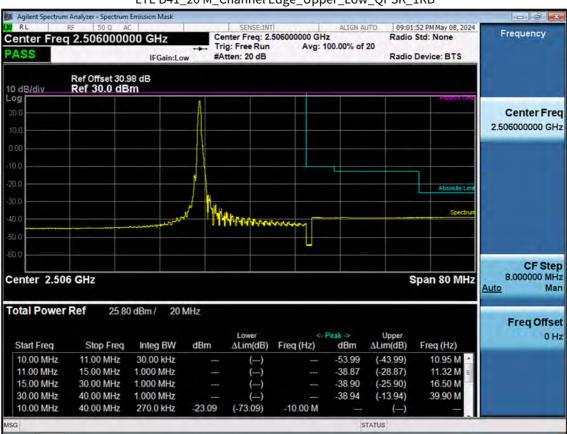
LTE B41\_20 M\_Channel Edge\_Upper\_Low\_QPSK\_1RB
