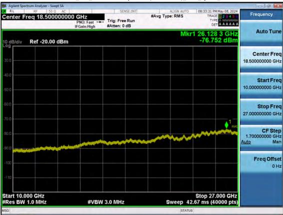
LTE B41\_5 M\_Conducted Spurious(Above10 G)\_Low\_QPSK\_1RB
