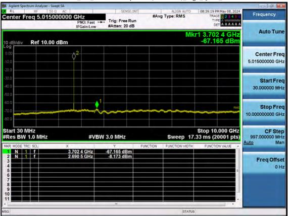
LTE B41\_5 M\_Conducted Spurious(30 M-10 G)\_High\_QPSK\_1RB
