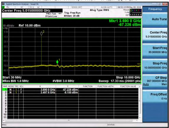
LTE B41\_15 M\_Conducted Spurious(30 M-10 G)\_Low\_QPSK\_1RB
