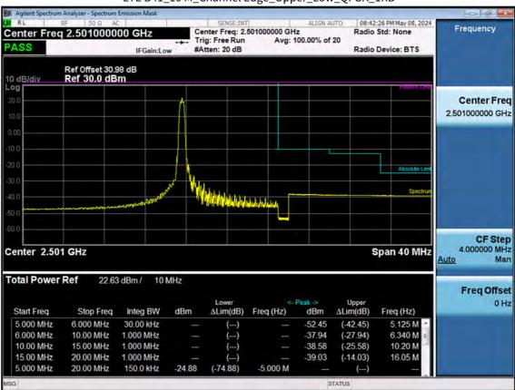
LTE B41\_10 M\_Channel Edge\_Upper\_Low\_QPSK\_1RB
