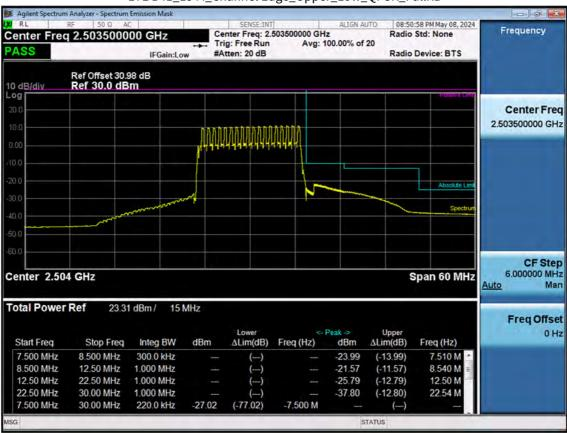
LTE B41\_15 M\_Channel Edge\_Upper\_Low\_QPSK\_FullRB
