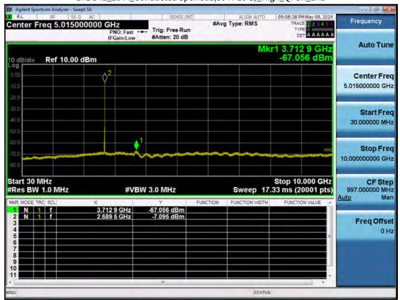
LTE B41\_20 M\_Conducted Spurious(30 M-10 G)\_High\_QPSK\_1RB
