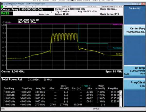
LTE B41\_20 M\_Channel Edge\_Upper\_Low\_QPSK\_FullRB
