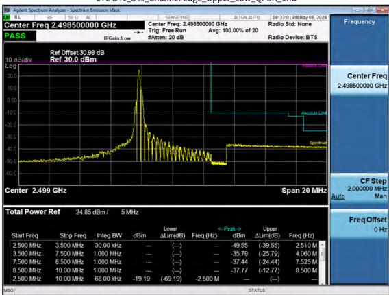
LTE B41\_5 M\_Channel Edge\_Upper\_Low\_QPSK\_1RB
