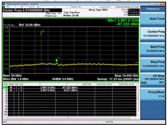
LTE B41\_20 M\_Conducted Spurious(30 M-10 G)\_Low\_QPSK\_1RB
