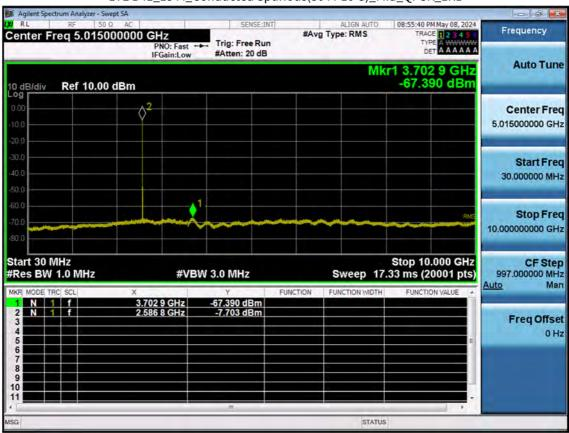
LTE B41\_15 M\_Conducted Spurious(30 M-10 G)\_Mid\_QPSK\_1RB
