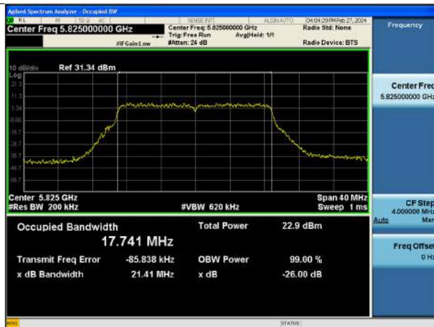
802.11ac(VHT40) 26 dB Bandwidth (CH 102)
