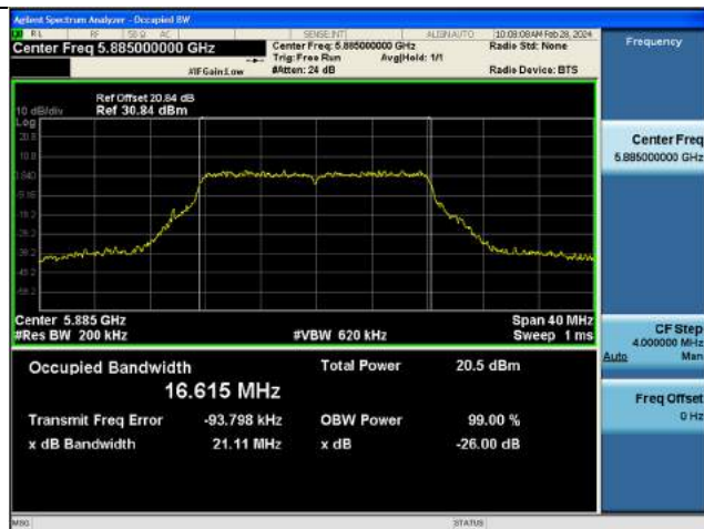
802.11ac(VHT20) 26 dB Bandwidth (CH 64)
