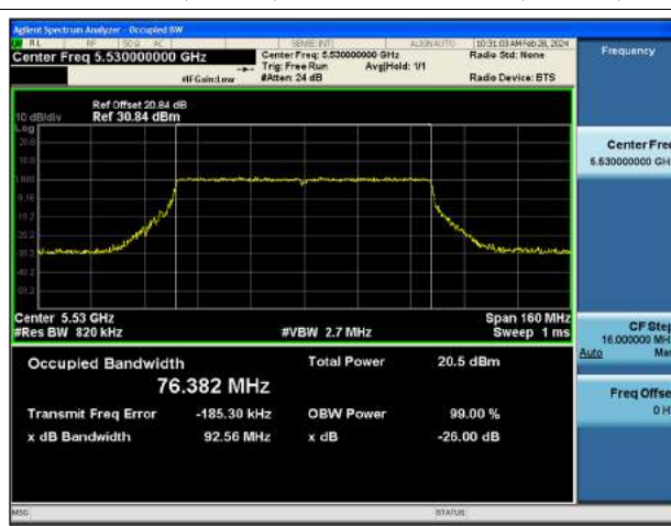
802.11ac(VHT80) 26 dB Bandwidth (CH 106)
