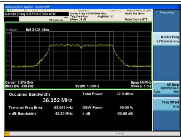
802.11ac(VHT80) 26 dB Bandwidth (CH 155)
