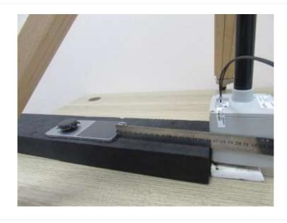
Edge 1 : 20 cm (The distance between the DUT and the center of the probe is 20 cm.)
