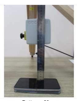
${\color{red}\textbf{Bottom: 20 cm}} \\ \text{(The distance between the DUT and the center of the probe is 20 cm.)}$
