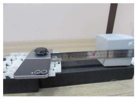
Edge 4:20 cm (The distance between the DUT and the center of the probe is 20 cm.)
