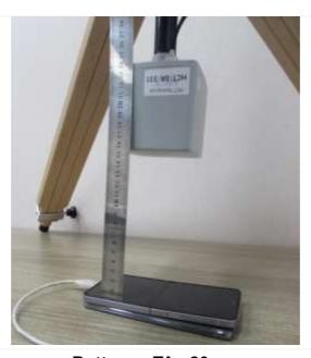
**Bottom + TA : 20 cm** (The distance between the DUT and the center of the probe is 20 cm.)
