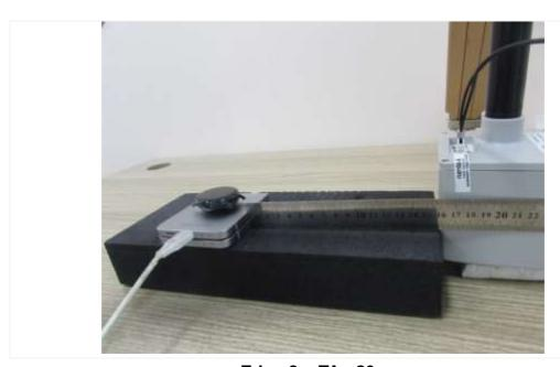
Edge 2 + TA : 20 cm (The distance between the DUT and the center of the probe is 20 cm.)
