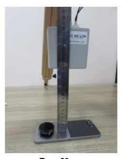
$\begin{tabular}{ll} \textbf{Top:20 cm} \\ \textbf{(The distance between the DUT and the center of the probe is 20 cm.)} \end{tabular}$
