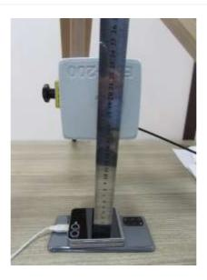
**Bottom + TA : 20 cm** (The distance between the DUT and the center of the probe is 20 cm.)
