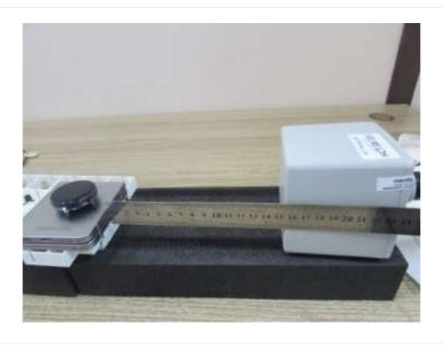
**Edge 2: 20 cm** (The distance between the DUT and the center of the probe is 20 cm.)
