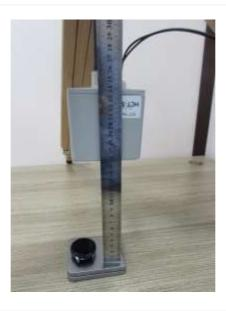
$\begin{tabular}{ll} \textbf{Top:20 cm} \\ \textbf{(The distance between the DUT and the center of the probe is 20 cm.)} \\ \end{tabular}$
