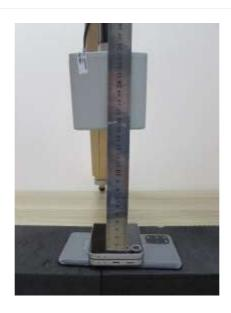
${\color{red}\textbf{Bottom: 20 cm}} \\ \text{(The distance between the DUT and the center of the probe is 20 cm.)}$
