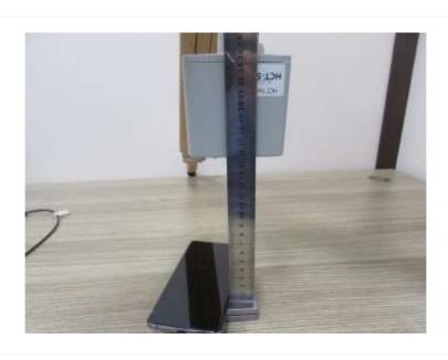
$\begin{tabular}{ll} \textbf{Top:20 cm} \\ \textbf{(The distance between the DUT and the center of the probe is 20 cm.)} \\ \end{tabular}$
