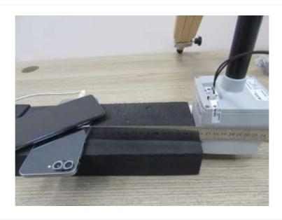
Edge 2 + TA : 20 cm (The distance between the DUT and the center of the probe is 20 cm.)
