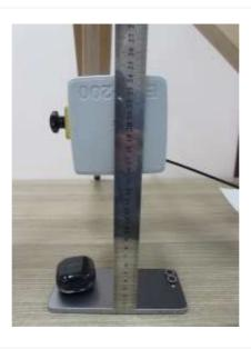
$\begin{tabular}{ll} \textbf{Top:20 cm} \\ \textbf{(The distance between the DUT and the center of the probe is 20 cm.)} \\ \end{tabular}$
