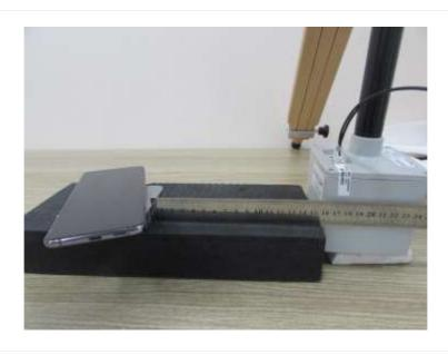
Edge 3:20 cm (The distance between the DUT and the center of the probe is 20 cm.)
