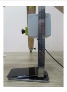
**Top: 20 cm** (The distance between the DUT and the center of the probe is 20 cm.)
