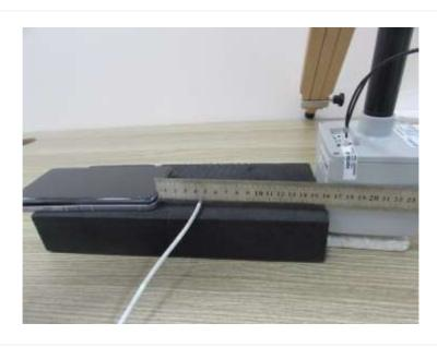
Edge 3 + TA : 20 cm (The distance between the DUT and the center of the probe is 20 cm.)
