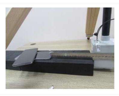
Edge 1 : 20 cm (The distance between the DUT and the center of the probe is 20 cm.)
