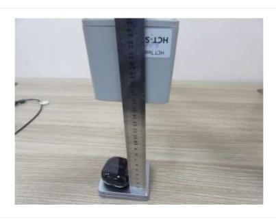
$\begin{tabular}{ll} \textbf{Top:20 cm} \\ \textbf{(The distance between the DUT and the center of the probe is 20 cm.)} \end{tabular}$
