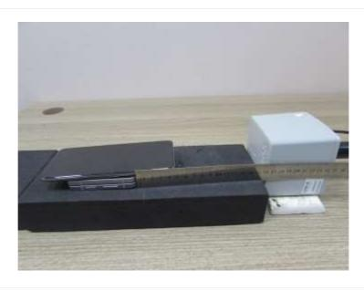
Edge 3:20 cm (The distance between the DUT and the center of the probe is 20 cm.)
