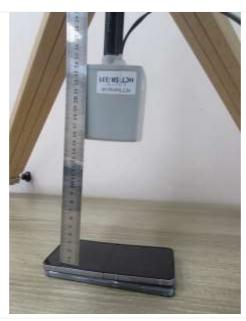
**Bottom: 20 cm** (The distance between the DUT and the center of the probe is 20 cm.)
