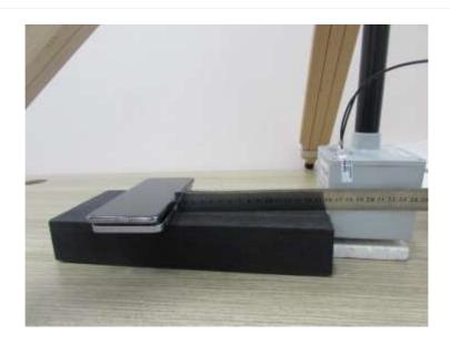
Edge 4:20 cm (The distance between the DUT and the center of the probe is 20 cm.)
