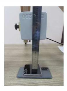
**Bottom : 20 cm** (The distance between the DUT and the center of the probe is 20 cm.)
