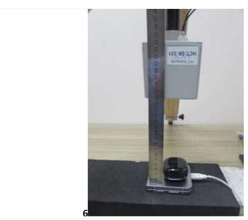
$\begin{tabular}{ll} \textbf{Top + TA : 20 cm} \\ \textbf{(The distance between the DUT and the center of the probe is 20 cm.)} \end{tabular}$
