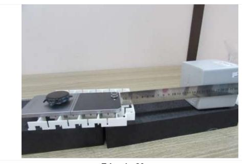
Edge 1 : 20 cm (The distance between the DUT and the center of the probe is 20 cm.)
