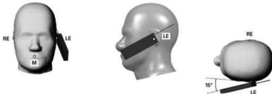
Figure 8.5. Tilt 15° position of the wireless device
