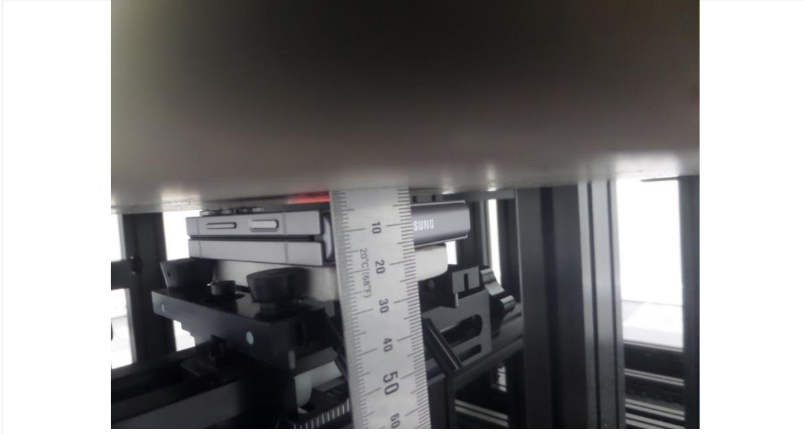
Distance of 5 mm from the EUT
