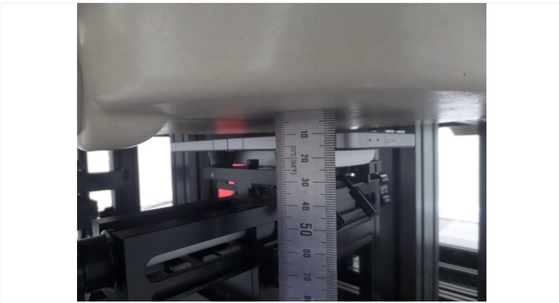
Distance of 10 mm from the EUT
