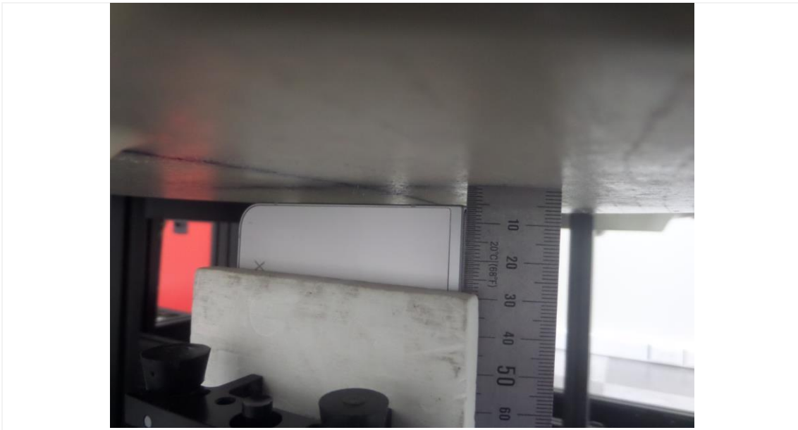
Distance of 5 mm from the EUT
