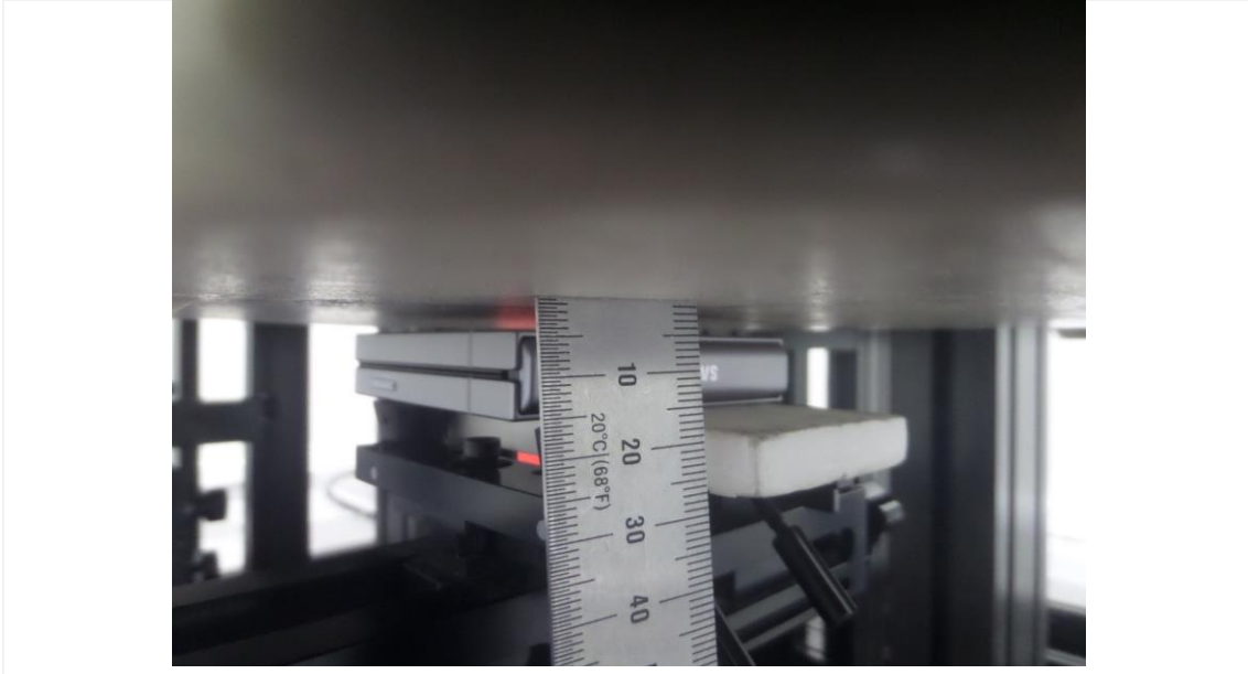
Distance of 5 mm from the EUT
