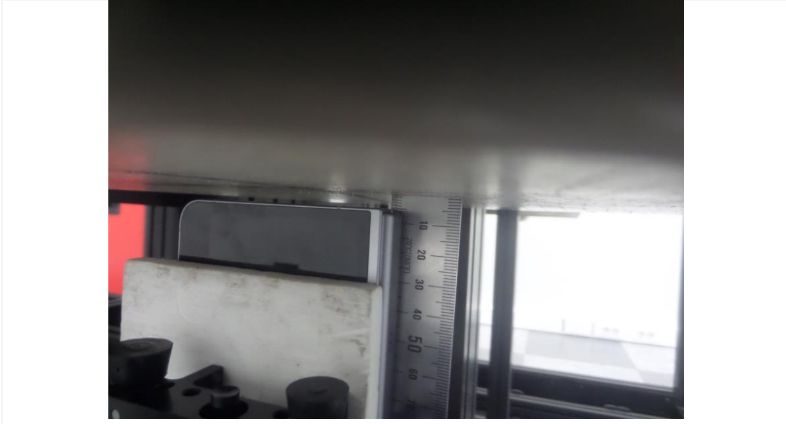
Distance of 5 mm from the EUT
