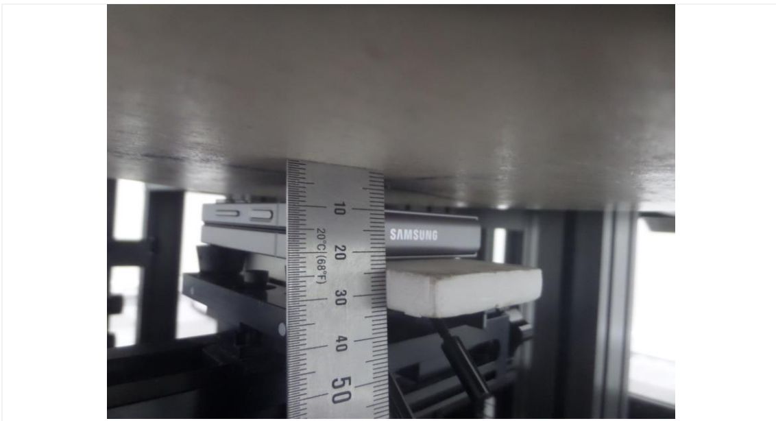
Distance of 10 mm from the EUT
