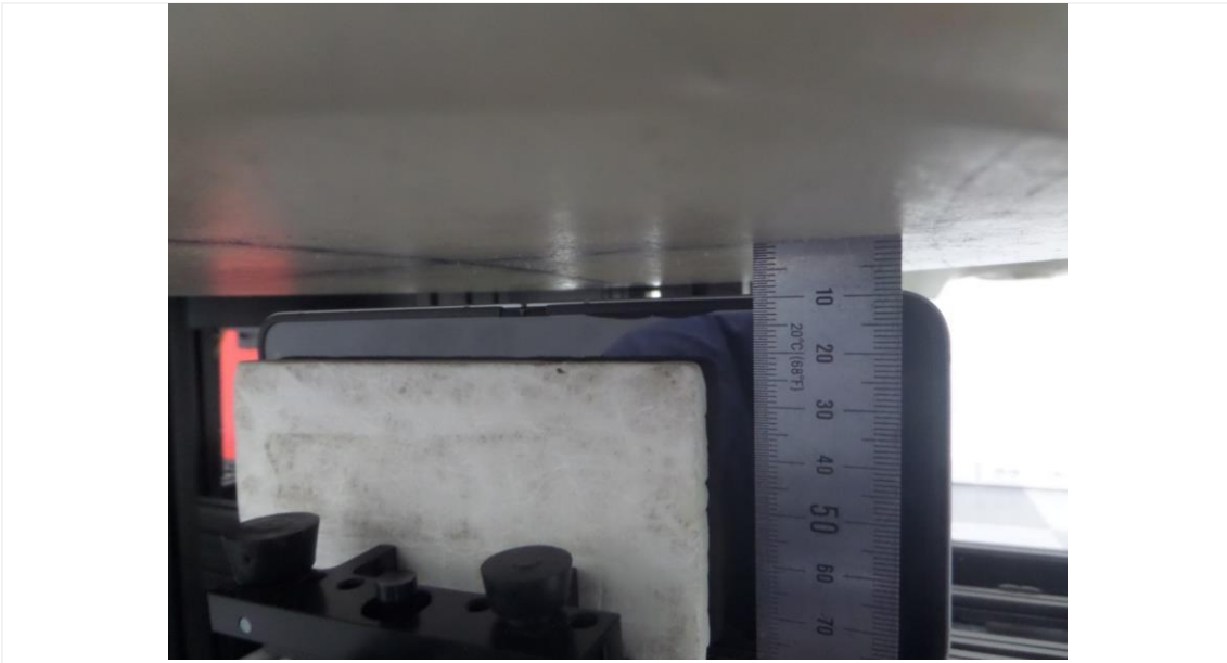
Distance of 10 mm from the EUT
