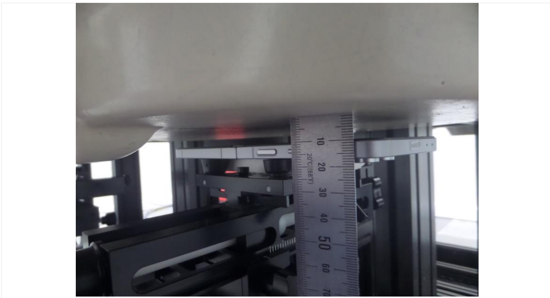
Distance of 10 mm from the EUT
