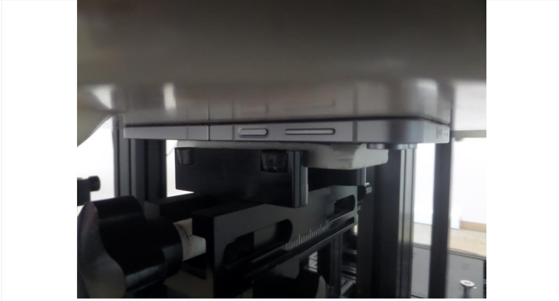
Distance of 0 mm from the EUT
