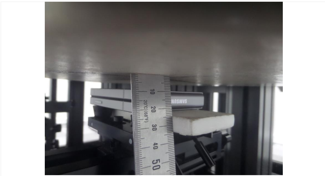
Distance of 10 mm from the EUT
