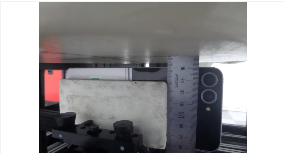
Distance of 10 mm from the EUT
