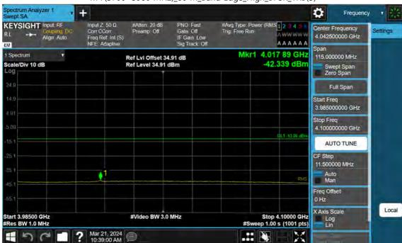
n77(3700~3980 MHz)\_80 M\_Band Edge\_High\_BPSK\_1RB(3)
