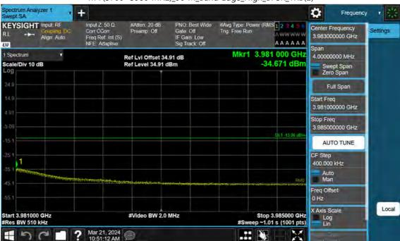
n77(3700~3980 MHz)\_90 M\_Band Edge\_High\_BPSK\_1RB(2)
