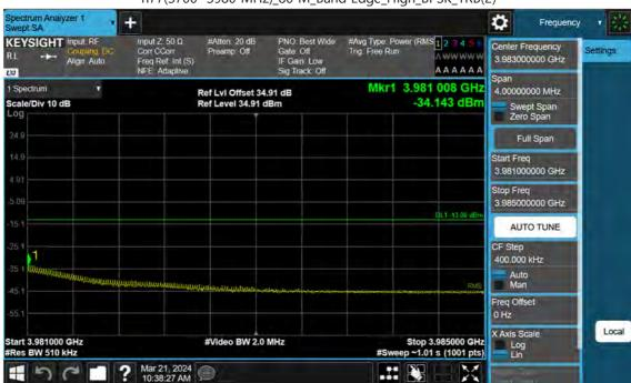
n77(3700~3980 MHz)\_80 M\_Band Edge\_High\_BPSK\_1RB(2)
