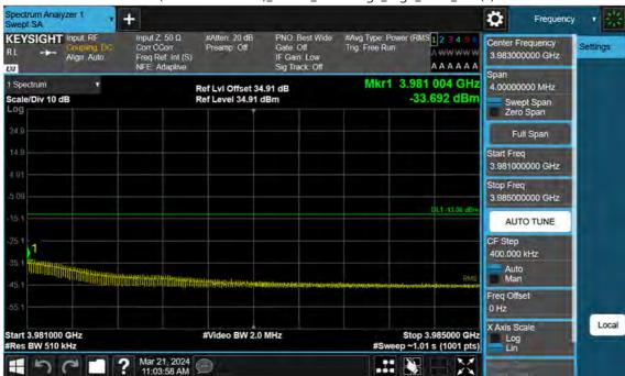
n77(3700~3980 MHz)\_100 M\_Band Edge\_High\_BPSK\_1RB(2)
