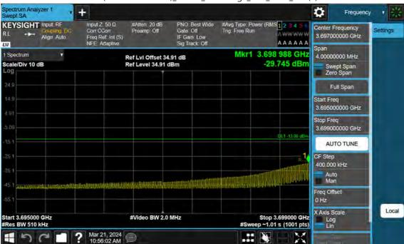
n77(3700~3980 MHz)\_100 M\_Band Edge\_Low\_BPSK\_1RB(2)
