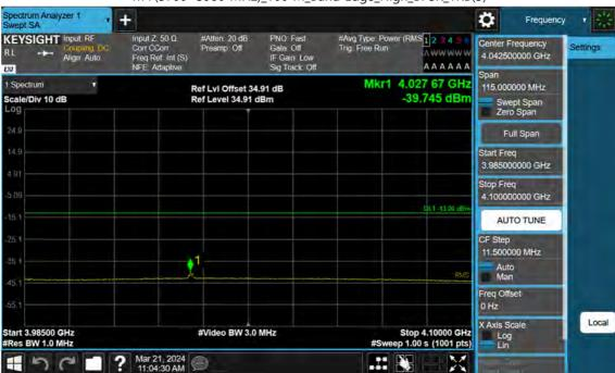
n77(3700~3980 MHz)\_100 M\_Band Edge\_High\_BPSK\_1RB(3)
