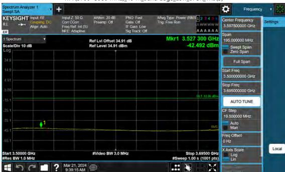
n77(3700~3980 MHz)\_40 M\_Band Edge\_Low\_BPSK\_1RB(3)
