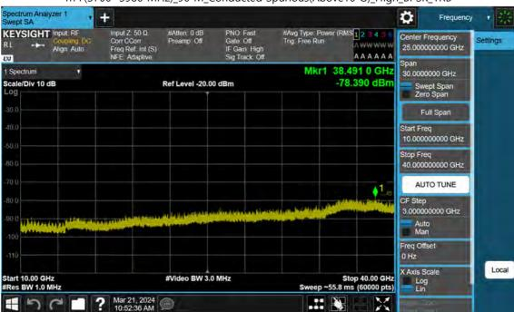
n77(3700~3980 MHz)\_90 M\_Conducted Spurious(Above10 G)\_High\_BPSK\_1RB
