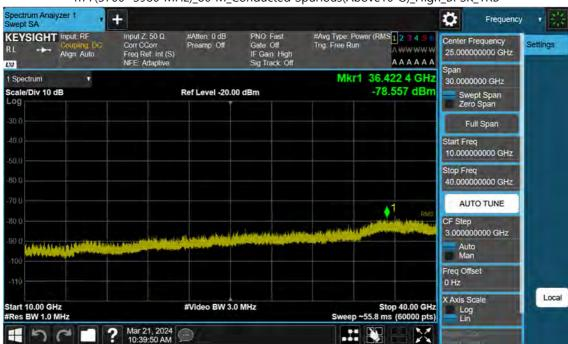
n77(3700~3980 MHz)\_80 M\_Conducted Spurious(Above10 G)\_High\_BPSK\_1RB
