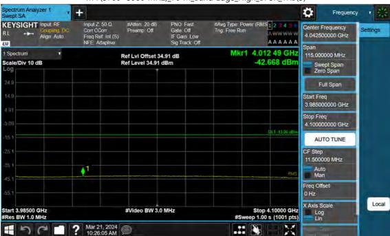
n77(3700~3980 MHz)\_70 M\_Band Edge\_High\_BPSK\_1RB(3)
