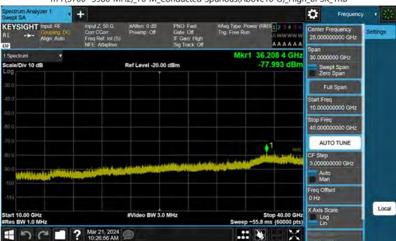
n77(3700~3980 MHz)\_70 M\_Conducted Spurious(Above10 G)\_High\_BPSK\_1RB
