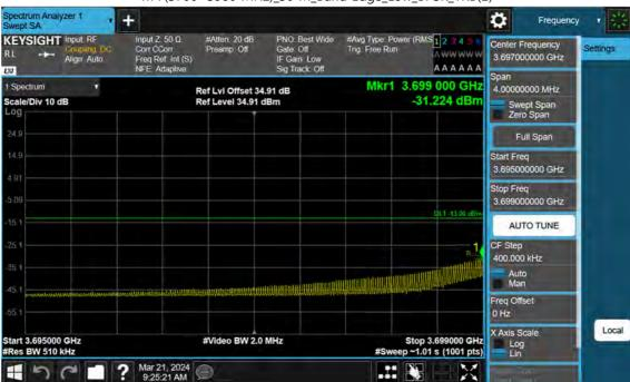
n77(3700~3980 MHz)\_30 M\_Band Edge\_Low\_BPSK\_1RB(2)
