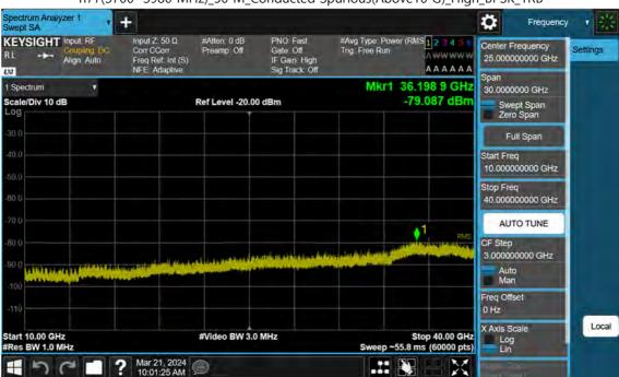
n77(3700~3980 MHz)\_50 M\_Conducted Spurious(Above10 G)\_High\_BPSK\_1RB
