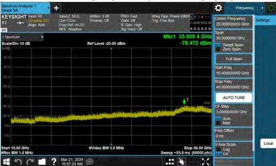
n77(3700~3980 MHz)\_100 M\_Conducted Spurious(Above10 G)\_Low\_BPSK\_1RB
