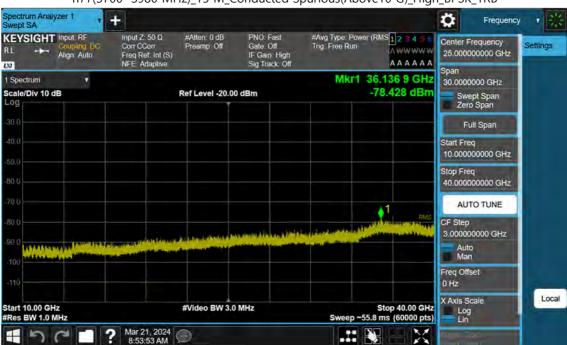
n77(3700~3980 MHz)\_15 M\_Conducted Spurious(Above10 G)\_High\_BPSK\_1RB
