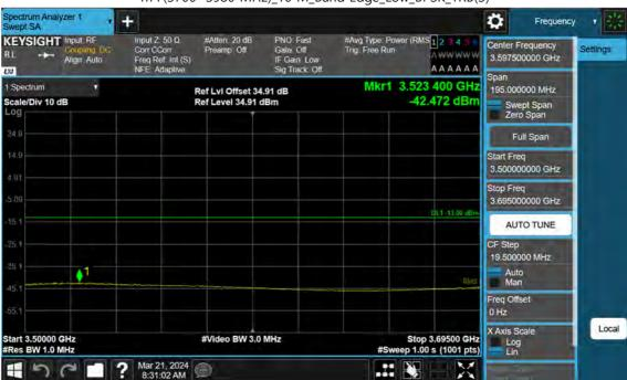
n77(3700~3980 MHz)\_10 M\_Band Edge\_Low\_BPSK\_1RB(3)
