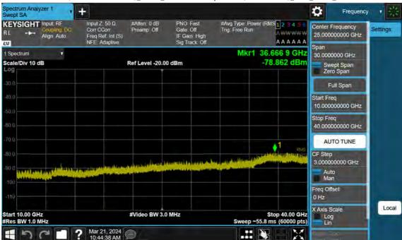
n77(3700~3980 MHz)\_90 M\_Conducted Spurious(Above10 G)\_Low\_BPSK\_1RB
