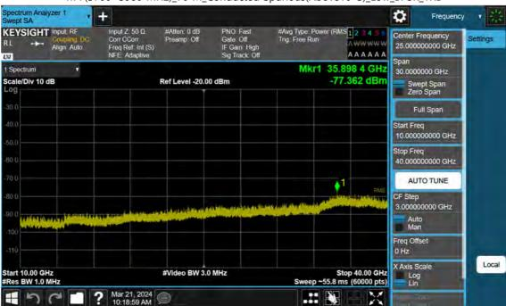
n77(3700~3980 MHz)\_70 M\_Conducted Spurious(Above10 G)\_Low\_BPSK\_1RB
