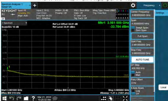
n77(3700~3980 MHz)\_70 M\_Band Edge\_High\_BPSK\_1RB(2)
