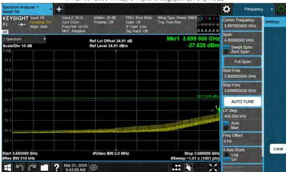
n77(3700~3980 MHz)\_15 M\_Band Edge\_Low\_BPSK\_1RB(2)
