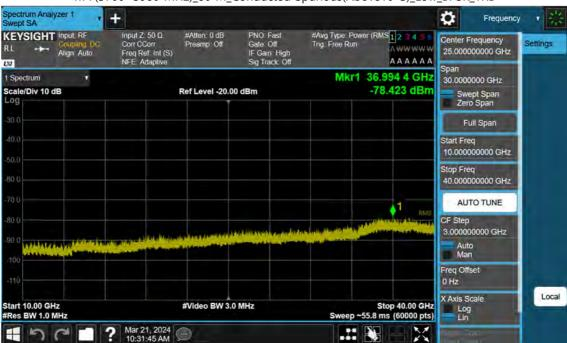
n77(3700~3980 MHz)\_80 M\_Conducted Spurious(Above10 G)\_Low\_BPSK\_1RB
