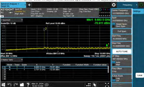
n77(3700~3980 MHz)\_90 M\_Conducted Spurious(30 M-10 G)\_Low\_BPSK\_1RB
