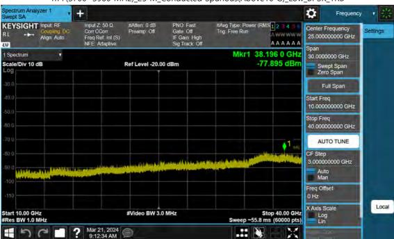
n77(3700~3980 MHz)\_25 M\_Conducted Spurious(Above10 G)\_Low\_BPSK\_1RB
