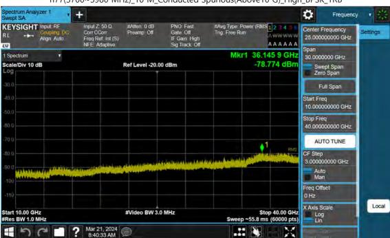
n77(3700~3980 MHz)\_10 M\_Conducted Spurious(Above10 G)\_High\_BPSK\_1RB
