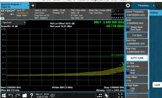
n77(3700~3980 MHz)\_40 M\_Band Edge\_Low\_BPSK\_1RB(2)
