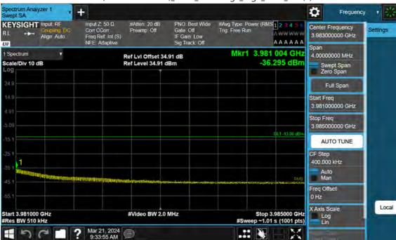
n77(3700~3980 MHz)\_30 M\_Band Edge\_High\_BPSK\_1RB(2)
