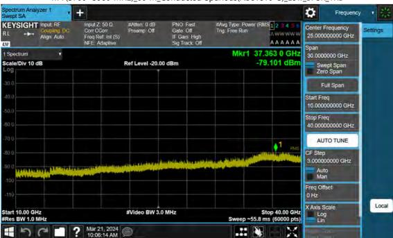
n77(3700~3980 MHz)\_60 M\_Conducted Spurious(Above10 G)\_Low\_BPSK\_1RB
