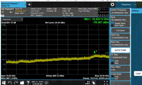
n77(3700~3980 MHz)\_40 M\_Conducted Spurious(Above10 G)\_High\_BPSK\_1RB
