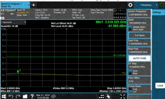
n77(3700~3980 MHz)\_15 M\_Band Edge\_Low\_BPSK\_1RB(3)
