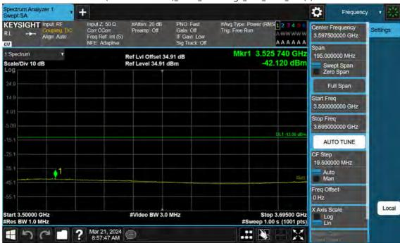
n77(3700~3980 MHz)\_20 M\_Band Edge\_Low\_BPSK\_1RB(3)
