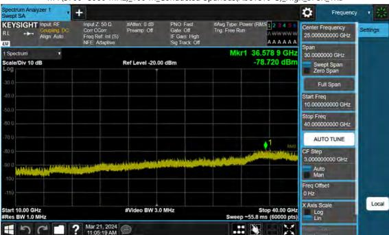
n77(3700~3980 MHz)\_100 M\_Conducted Spurious(Above10 G)\_High\_BPSK\_1RB
