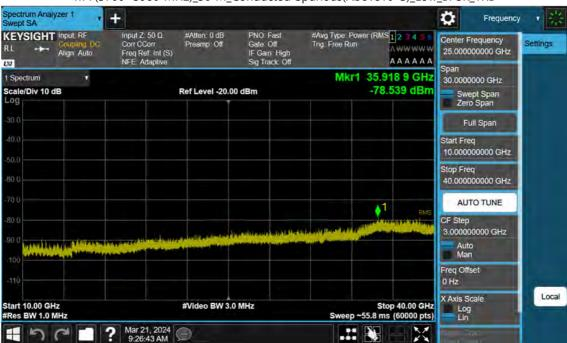
n77(3700~3980 MHz)\_30 M\_Conducted Spurious(Above10 G)\_Low\_BPSK\_1RB
