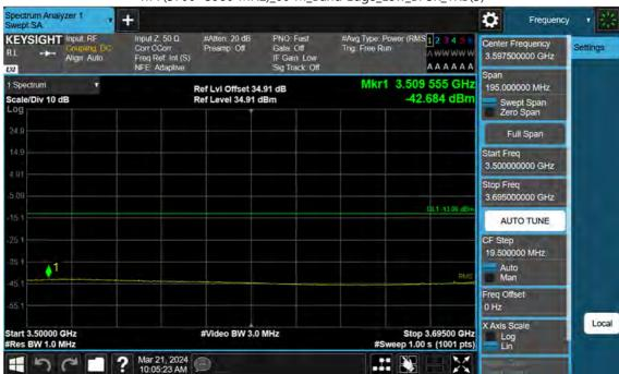
n77(3700~3980 MHz)\_60 M\_Band Edge\_Low\_BPSK\_1RB(3)
