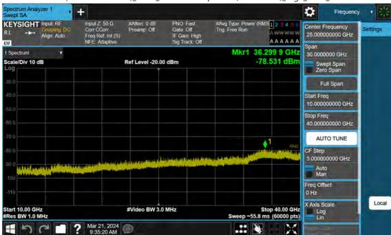
n77(3700~3980 MHz)\_30 M\_Conducted Spurious(Above10 G)\_High\_BPSK\_1RB
