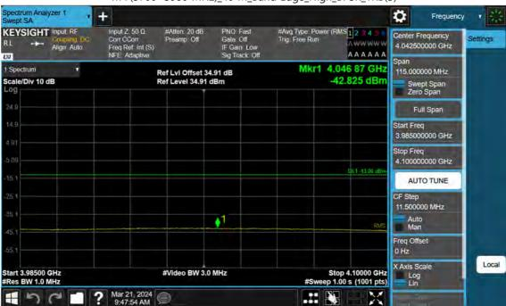
n77(3700~3980 MHz)\_40 M\_Band Edge\_High\_BPSK\_1RB(3)
