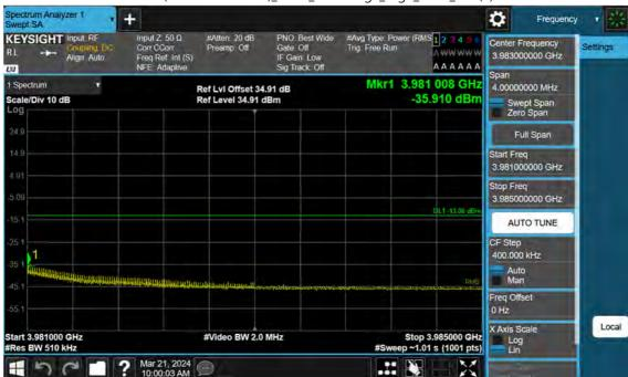
n77(3700~3980 MHz)\_50 M\_Band Edge\_High\_BPSK\_1RB(2)
