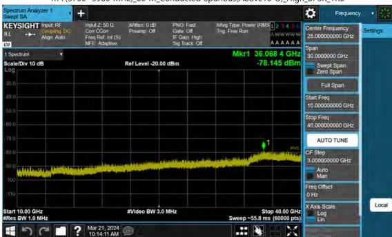
n77(3700~3980 MHz)\_60 M\_Conducted Spurious(Above10 G)\_High\_BPSK\_1RB
