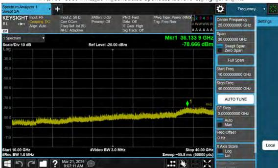
n77(3700~3980 MHz)\_20 M\_Conducted Spurious(Above10 G)\_High\_BPSK\_1RB
