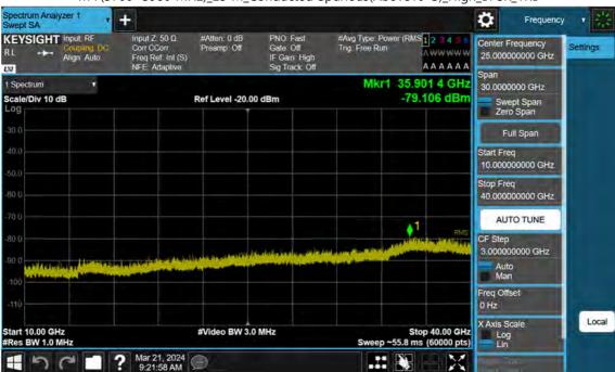
n77(3700~3980 MHz)\_25 M\_Conducted Spurious(Above10 G)\_High\_BPSK\_1RB
