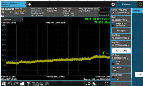
n77(3700~3980 MHz)\_50 M\_Conducted Spurious(Above10 G)\_Low\_BPSK\_1RB
