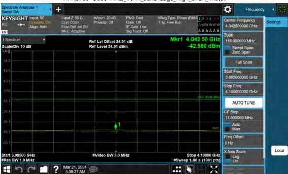
n77(3700~3980 MHz)\_10 M\_Band Edge\_High\_BPSK\_1RB(3)
