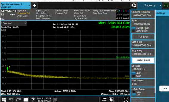
n77(3700~3980 MHz)\_60 M\_Band Edge\_High\_BPSK\_1RB(2)
