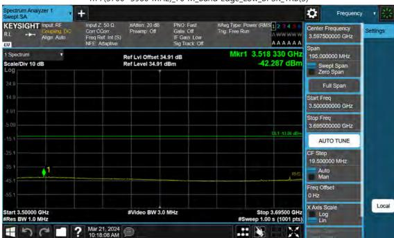
n77(3700~3980 MHz)\_70 M\_Band Edge\_Low\_BPSK\_1RB(3)
