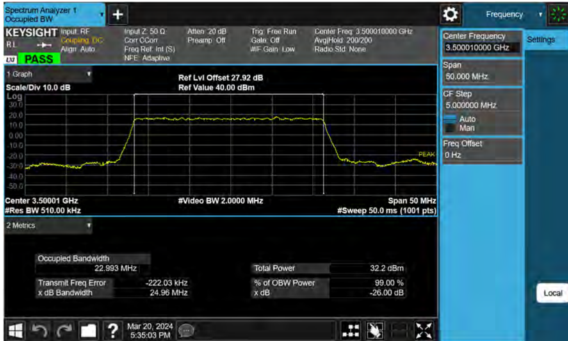
n77(3450~3550 MHz)_25 M_OBW_Mid_BPSK_FullIRB
