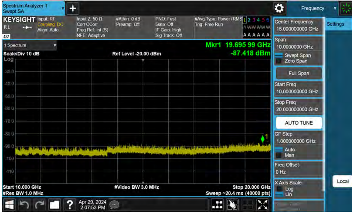
Sub6 n25(2)_25 M_Conducted Spurious(Above10 G)_High_BPSK_1RB
