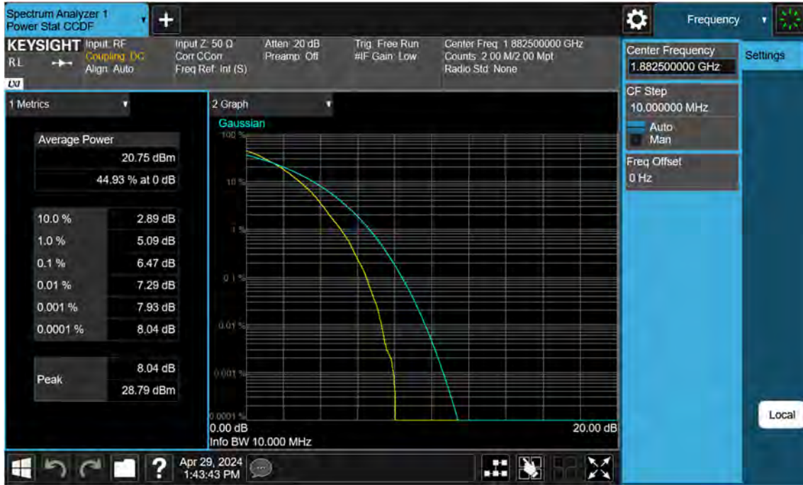
Sub6 n25(2)_10 M_PAR_Mid_256QAM_FullRB
