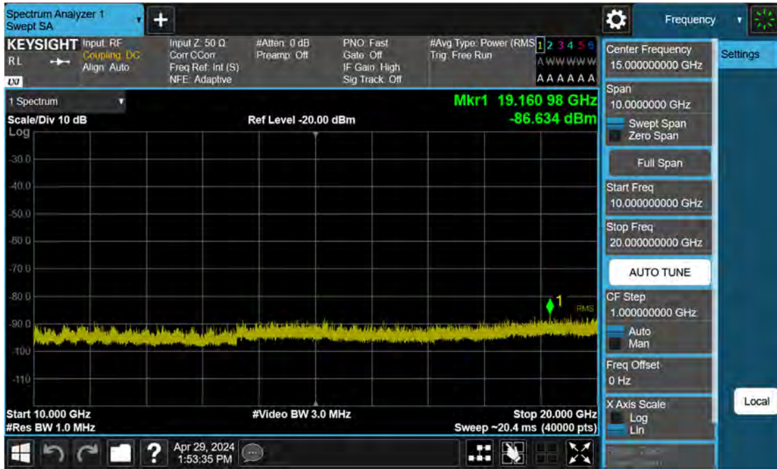
Sub6 n25(2)_15 M_Conducted Spurious(Above10 G)_High_BPSK_1RB
