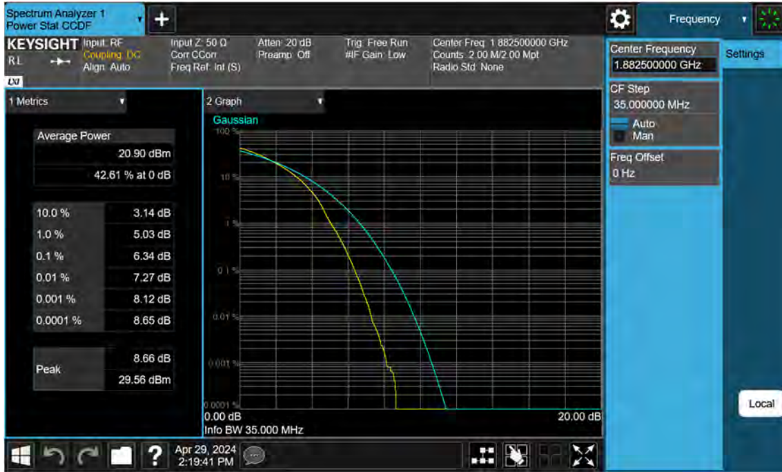
Sub6 n25(2)_35 M_PAR_Mid_256QAM_FullRB
