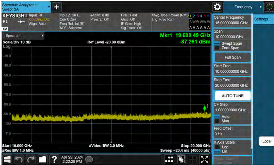
Sub6 n25(2)_35 M_Conducted Spurious(Above10 G)_High_BPSK_1RB
