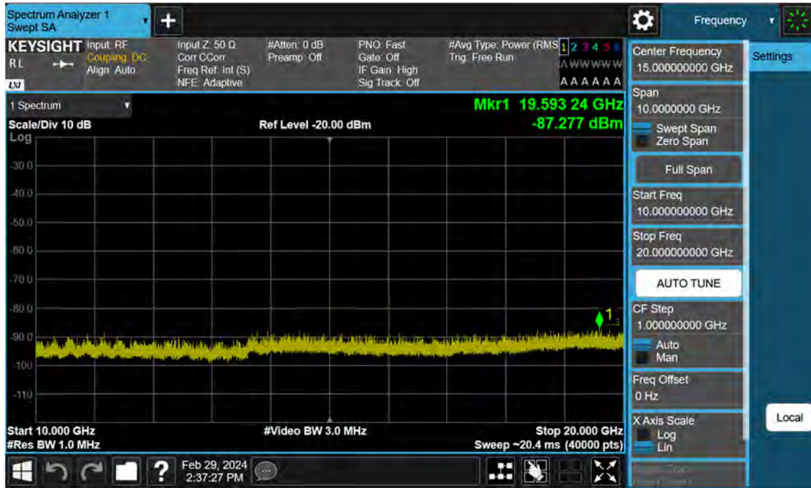
Sub6 n25_15 M_Conducted Spurious(Above10 G)_Low_BPSK_1RB
