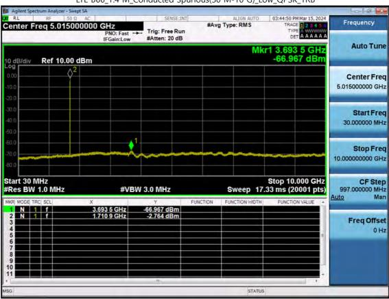
LTE B66\_1.4 M\_Conducted Spurious(30 M-10 G)\_Low\_QPSK\_1RB
