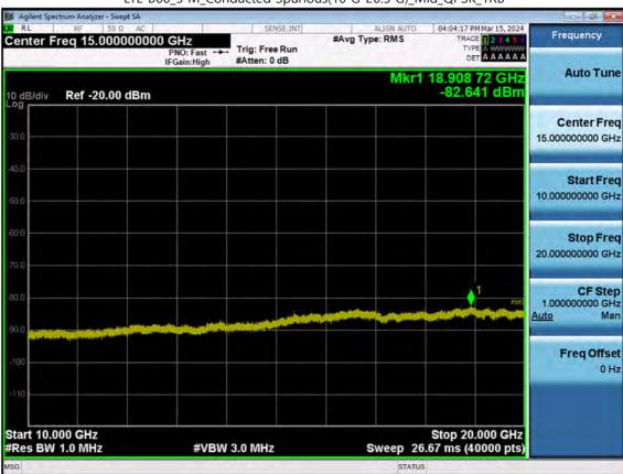
LTE B66\_5 M\_Conducted Spurious(10 G-26.5 G)\_Mid\_QPSK\_1RB
