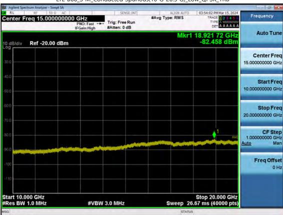
LTE B66\_3 M\_Conducted Spurious(10 G-26.5 G)\_Low\_QPSK\_1RB
