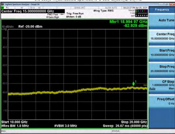
LTE B25\_3 M\_Conducted Spurious(10 G-26.5 G)\_Low\_QPSK\_1RB
