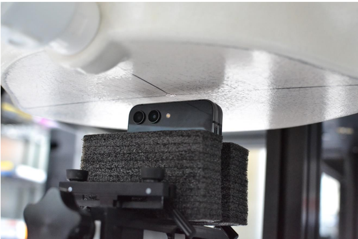
SAR Test Setup Photo 12 – Closed Hotspot, Bottom Edge at 5 mm
