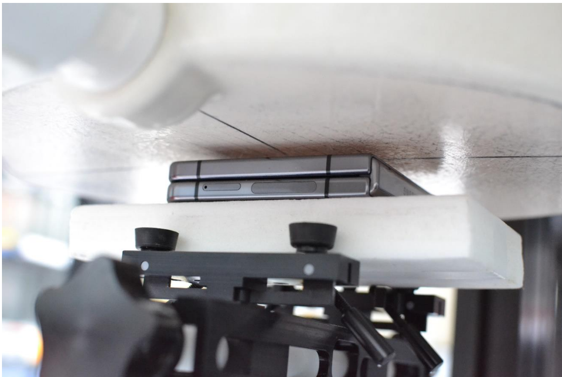
SAR Test Setup Photo 10 – Closed Hotspot, Back Side at 5 mm
