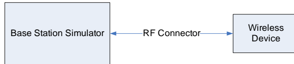
Figure 9-1 Power Measurement Setup – NR FDD
