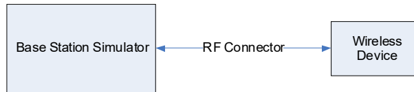
Figure 9-3 Power Measurement Setup
