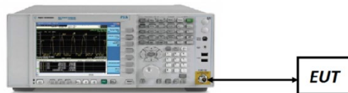
Figure 7-3. Test Instrument & Measurement Setup
