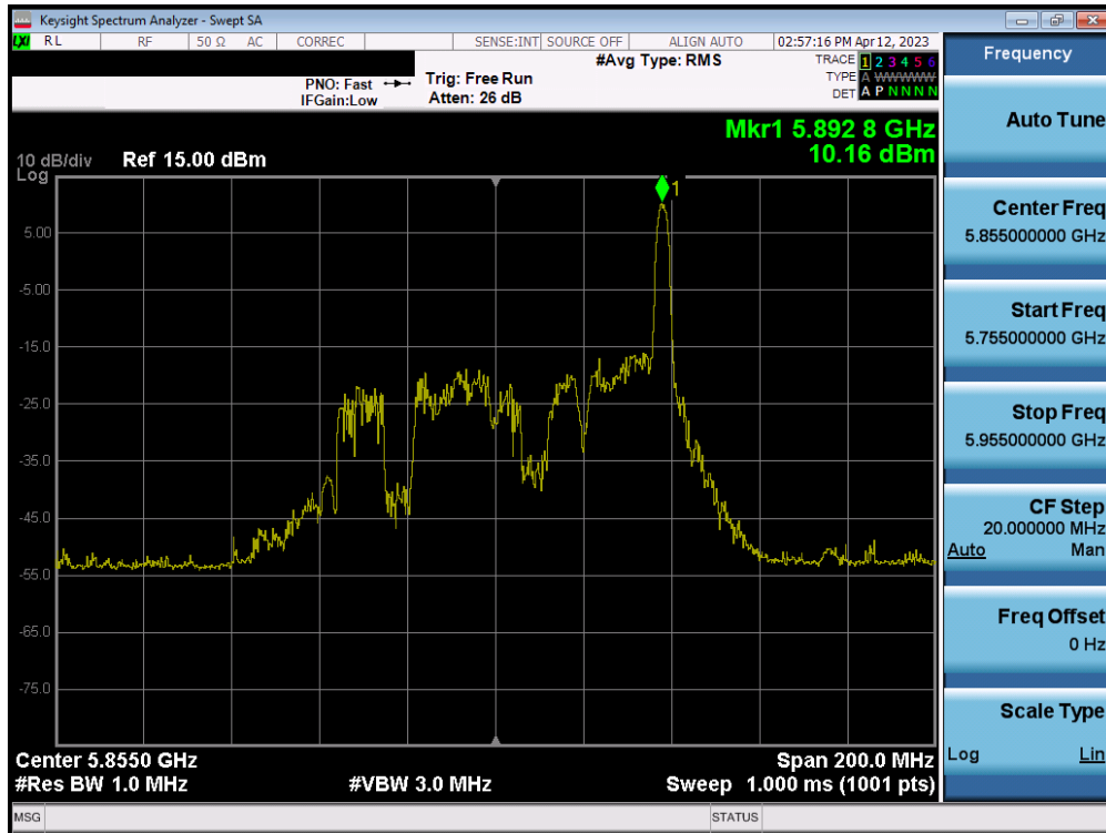
Plot 7-125. Power Spectral Density Plot MIMO ANT2 (80MHz BW 802.11ax – 26 Tones (UNII Band 3/4) – Ch. 171)
