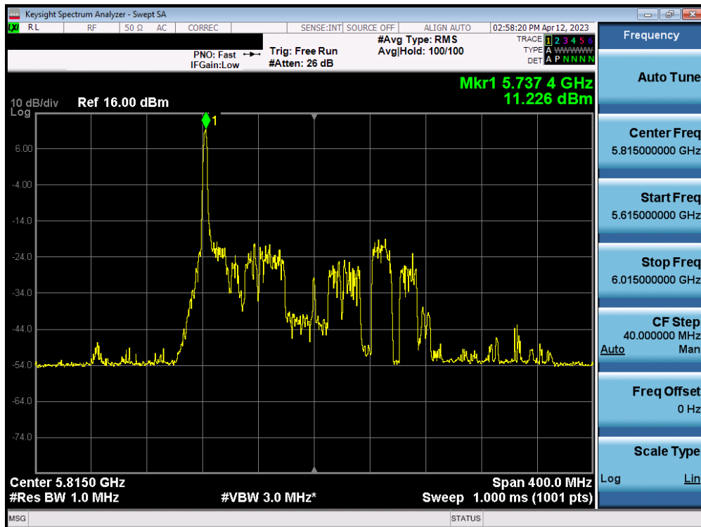
Plot 7-126. Power Spectral Density Plot MIMO ANT2 (160MHz BW 802.11ax – 26 Tones (UNII Band 3/4) – Ch. 163)
