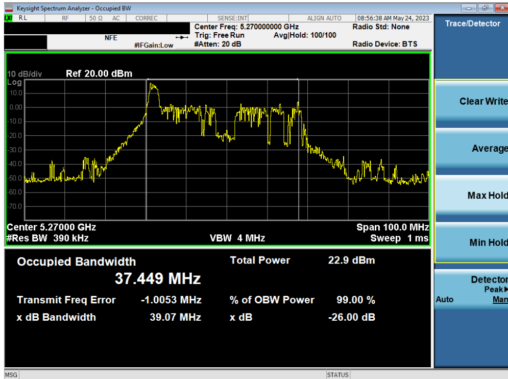
Plot 7-6. 26dB Bandwidth Plot MIMO ANT1 (40MHz BW 802.11ax – 26 Tones (UNII Band 2A) – Ch. 54)
