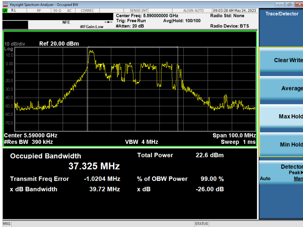
Plot 7-9. 26dB Bandwidth Plot MIMO ANT1 (40MHz BW 802.11ax – 26 Tones (UNII Band 2C) – Ch. 118)
