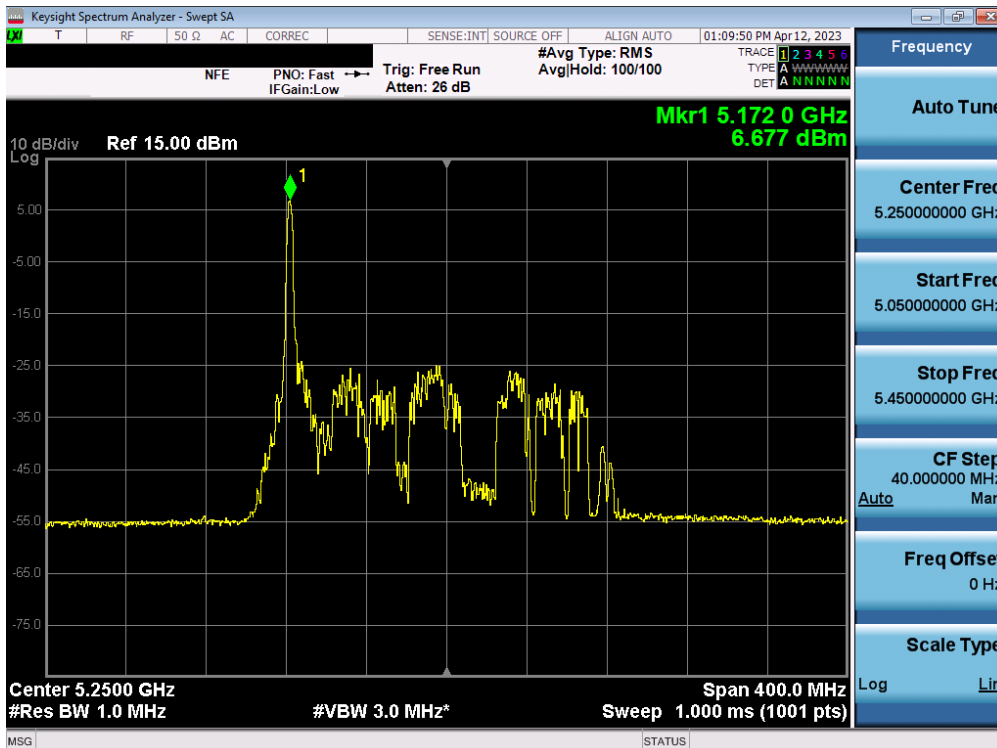
Plot 7-76. Power Spectral Density Plot MIMO ANT1 (160MHz BW 802.11ax – 26 Tones (UNII Band 1/2A) – Ch. 50)
